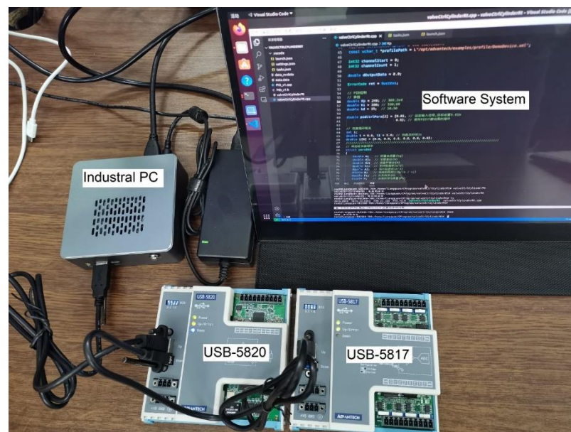
Figure 9. Physical HIL simulation system prototype.
