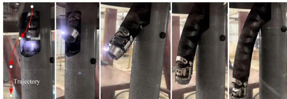
Figure 11. Trajectory for passing through the divider plug.
