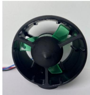
**Figure 8.** The thruster of AUV.
