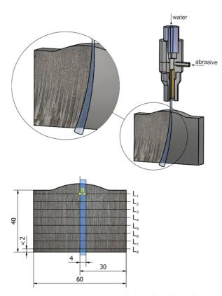
**Figure 4.** Measurement principle, displayed lines from L1 to L8, direction of travel of the roughness measuring probe (measured length  $l_r = 4$  mm, direction of tip movement—in the direction of the arrow "a"), and the actual surface after the AWJ machining (sample 1, set Q1).
