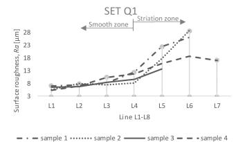
Figure 5. Evaluation of surface topography created by the AWJ (set Q1).
