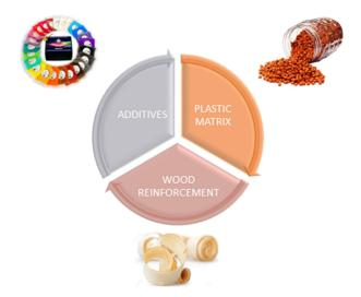
Figure 1. Wood-filled plastic components [31–33].
