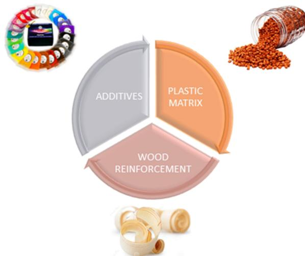
**Figure 1.** Wood-filled plastic components [31–33].
