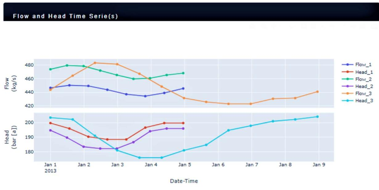
**Figure 12.** The user interface used to drive operational consequence decision support tool: trajectory is converted into flow and head time series.
