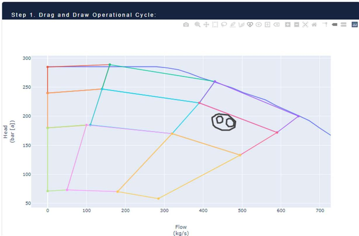
**Figure 11.** The user interface used to drive operational consequence decision support tool: Operator ‘draws’ (black line) anticipated trajectory across pump curve representation.
