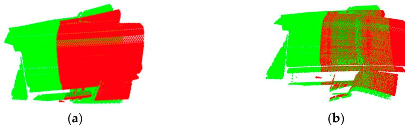
**Figure 21.** Comparison of the overall stitching effect of the vehicle nose. (a) Initial point cloud stitching. (b) DeepMerge algorithm correction.
