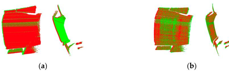
**Figure 22.** Comparison of the effect of one stitching at the same position. (a) Initial point cloud stitching. (b) DeepMerge algorithm correction.
