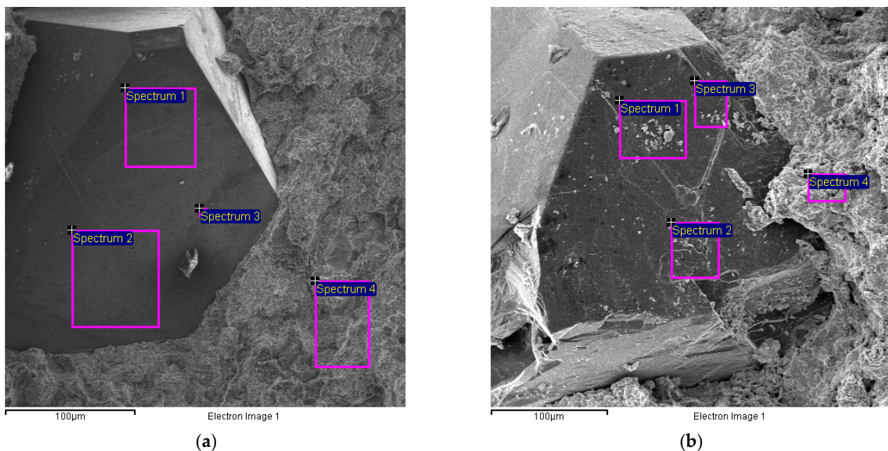
Figure 6. SEM images of sintered samples microstructure, obtained under the composite contrast, showing EDS areas: (a) Sample 1; (b) Sample 5.
