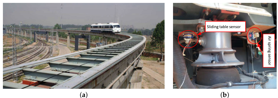
Figure 8. Test on circular curve. (a) Maglev train running on R100m circular curve on the Tangshan test line; (b) sensor for displacement test of sliding table and air spring.
