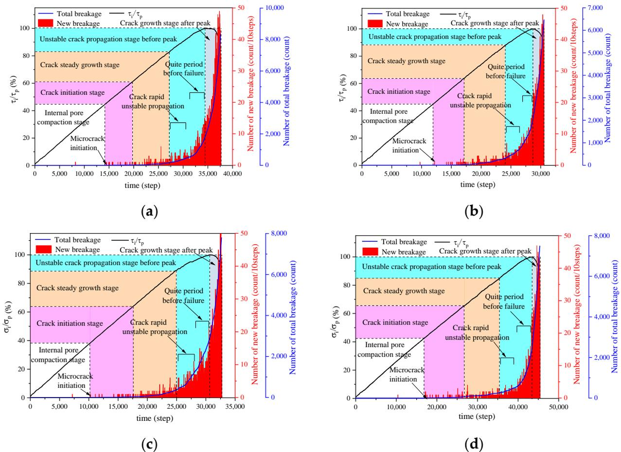
**Figure 15.** Variation of breakage number with time steps in the loading process of the model: (a) Positive shear; (b) Reverse shear; (c) Lateral shear; (d) Intact sample shear.
