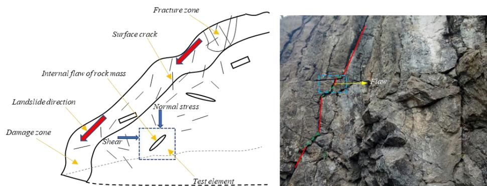
**Figure 1.** Stress diagram of high defect rock slope.
