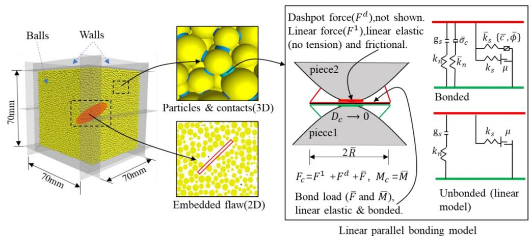
Figure 11. PFC3D model sample and parallel bonding model.
