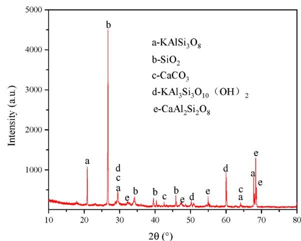
**Figure 4.** X-diffraction of the rock-like sample.
