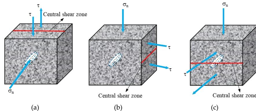
**Figure 5.** Schematic diagram of a sample with flaw shear in three different directions (taking an angle  $\alpha = 45^\circ$  as an example): (a) Positive shear; (b) Reverse shear; (c) Lateral shear.
