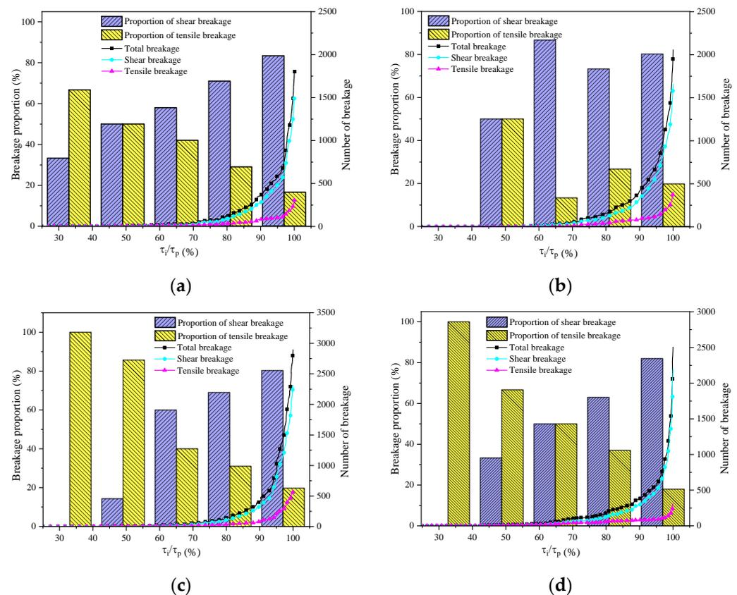
**Figure 16.** Variation law of the proportion of tensile shear breaking number with the increase in shear stress: (a) Positive shear; (b) Reverse shear; (c) Lateral shear; (d) Intact sample shear.
