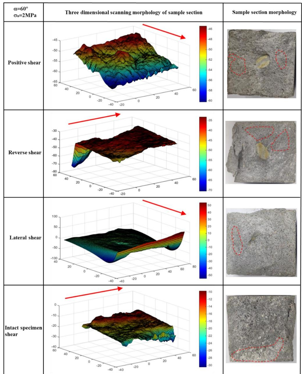
**Figure 9.** Comparison of 3D scanning morphology characteristics of sections from each sample after failure ( $\sigma_n = 2 \text{ MPa}$ ,  $\alpha = 60^\circ$ ).
