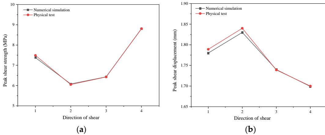
**Figure 12.** Comparison between peak parameters of the four groups of model samples and physical test results: (a) peak shear strength; (b) peak shear displacement.
