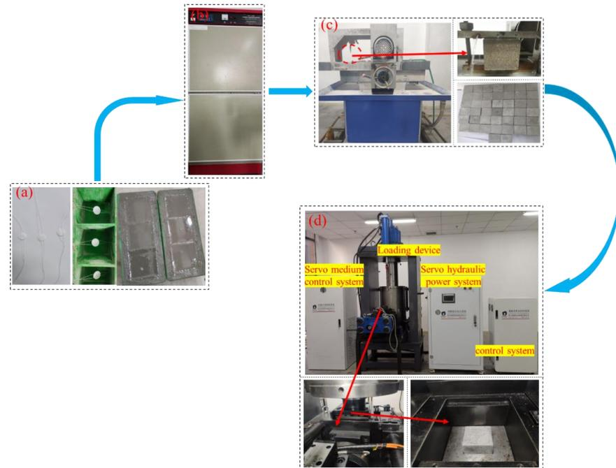
**Figure 3.** Sample preparation and shear test equipment: (a) preparation of the samples before pouring; (b) constant temperature and humidity curing box; (c) sample grinding process; (d) mechanical loading equipment.
