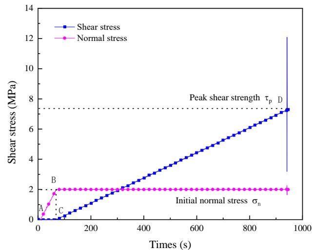
Figure 6. Schematic diagram of sample loading path.
