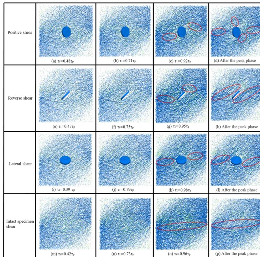
Figure 18. Changes in contact force chain of four groups of model samples at different stages.
