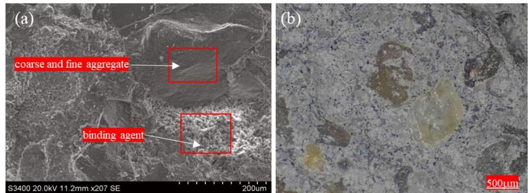
Figure 10. Microstructure of rock materials: (a) scanning electron microscope (SEM) image; (b) cross-section light microscope image.
