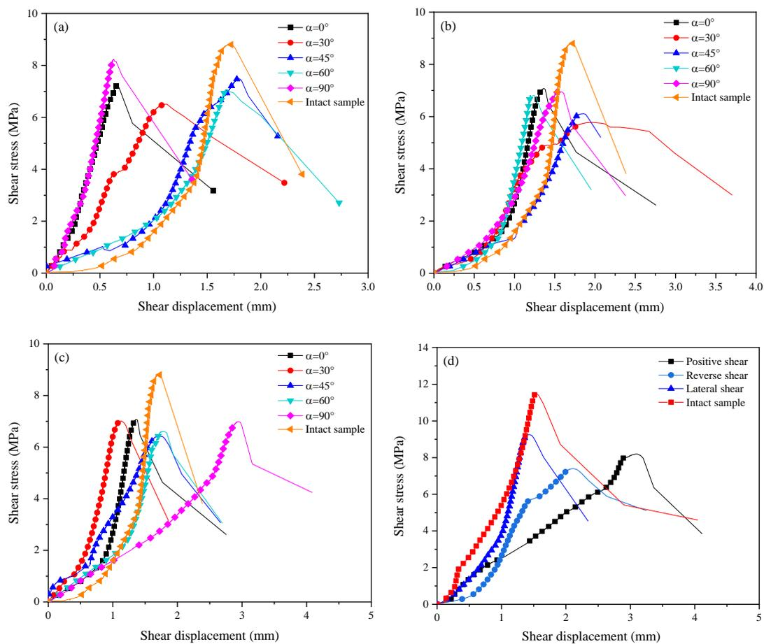
**Figure 7.** Shear stress-shear displacement curve: (a) positive shear,  $\sigma_n = 2$  MPa; (b) reverse shear,  $\sigma_n = 2$  MPa; (c) lateral shear,  $\sigma_n = 2$  MPa; (d)  $\alpha = 45^\circ$ ,  $\sigma_n = 4$  MPa.
