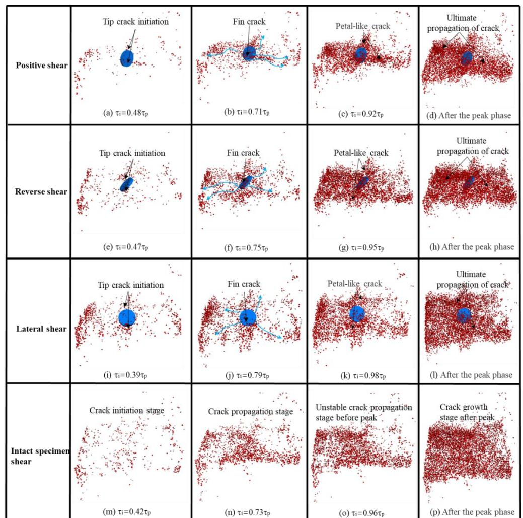
Figure 14. Microcrack propagation of four groups of models in different servo loading stages.
