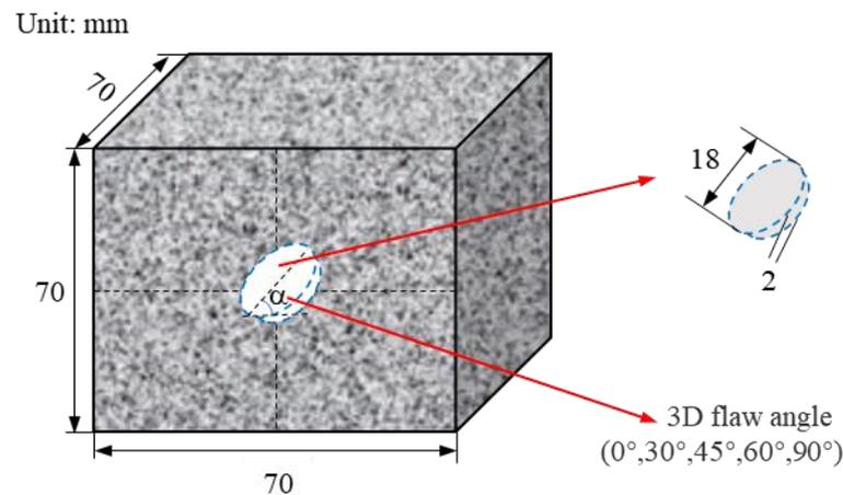
**Figure 2.** Sample size and flaw geometric parameters.
