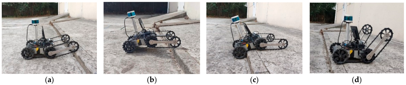
Figure 11. Robot climbing up steps: (a) lift the rocker arm; (b) track wheels against the step; (c) centroid crossing the step; (d) car body over the step.
