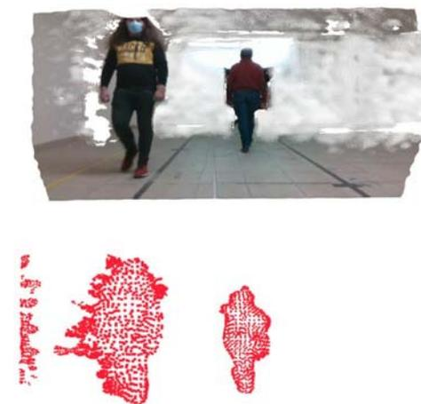
**Figure 5.** Moving obstacle detection (pedestrians walking in opposite directions). In this test, the AGV was stationary. **(Top)**: original point cloud; **(Bottom)**: detected clusters.
