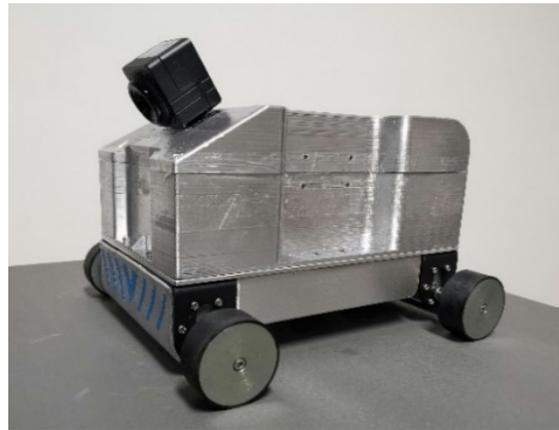
**Figure 2.** Prototype of the wall-climbing robot.
