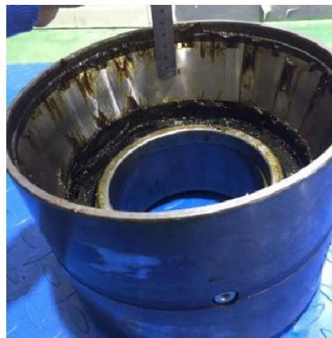
Figure 18. Weak fault morphology and the dimension of the outer ring of the axle box bearing.
