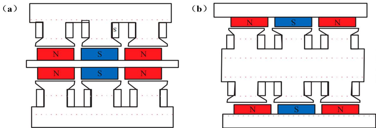
**Figure 4.** The topological structures of AFIR and TORUS: (a) AFIR type; (b) TORUS type. Adapted from Ref. [31]. Copyright 2018 MDPI.
