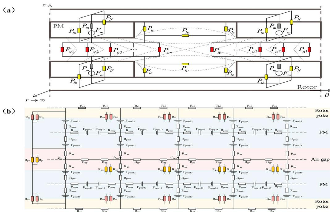
**Figure 7.** Electromagnetic modeling of MEC. (a) 3-D MEC model considering magnetic leakage and fringing flux. Adapted with permission from Ref. [75]. Copyright 2021 John Wiley and Sons. (b) MEC model considering end leakage fluxes. Adapted with permission from Ref. [76]. Copyright 2019 John Wiley and Sons.
