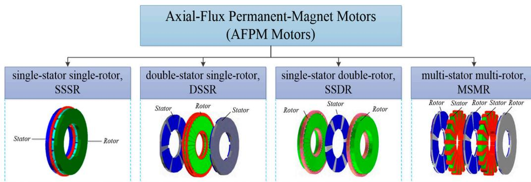
**Figure 3.** Four typical types of topological structures of AFPM motors.
