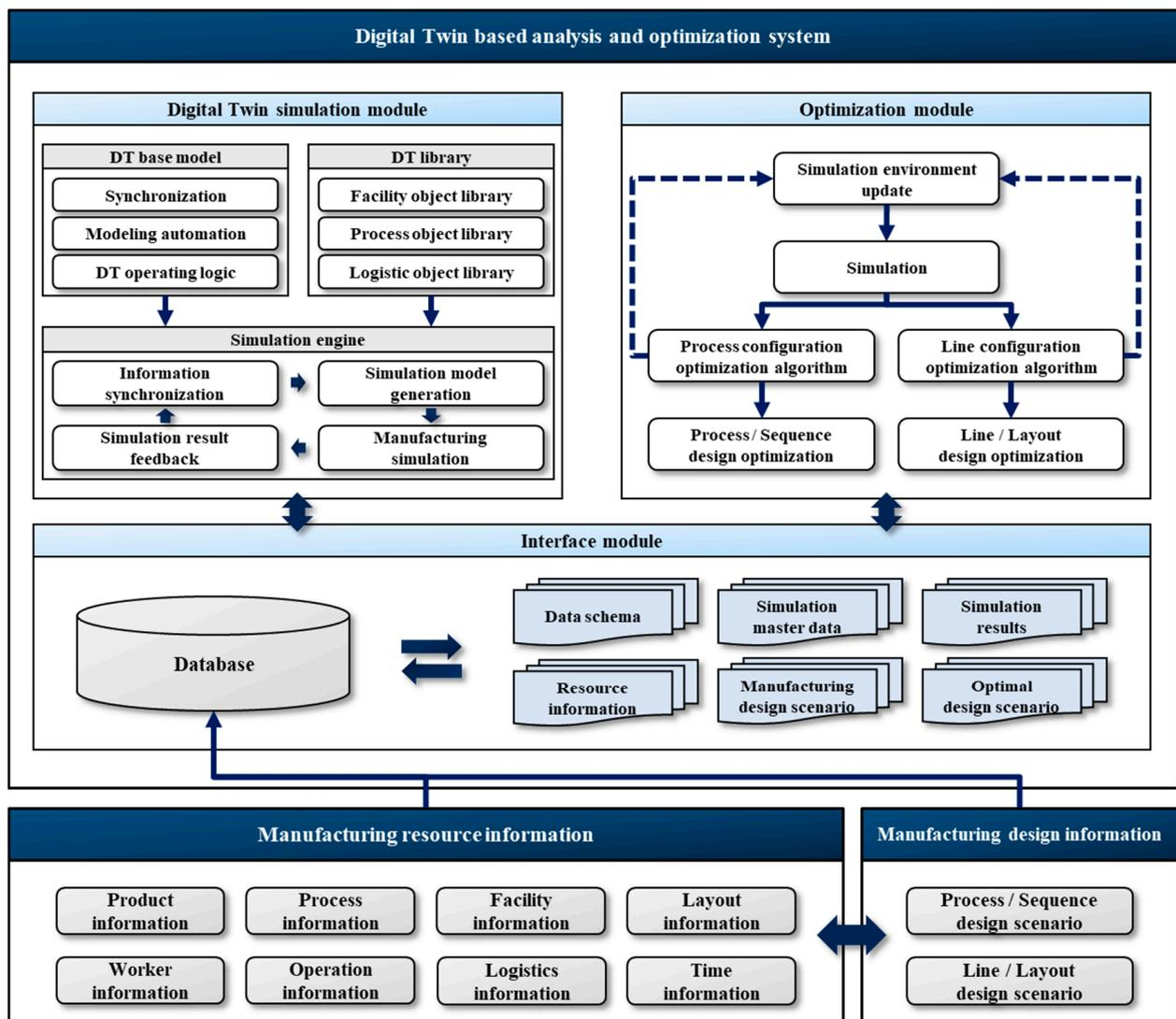
Figure 1. Framework for the DT-based analysis and optimization system.
