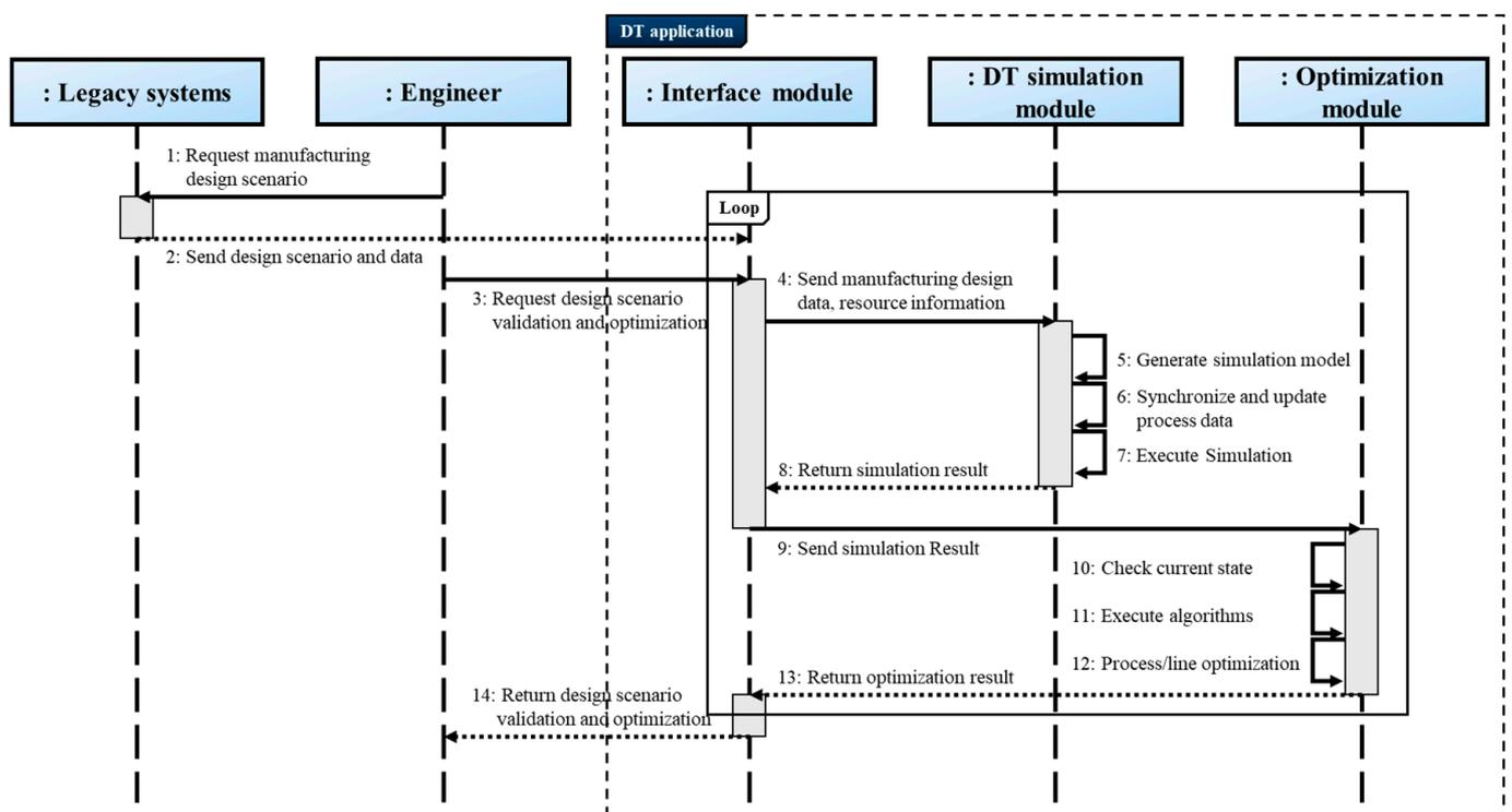
**Figure 2.** Operation procedure of DT application.
