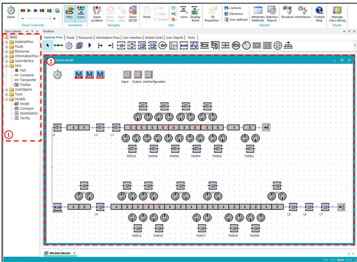
Figure 4. Example of the implemented DT simulation module and simulation model.
