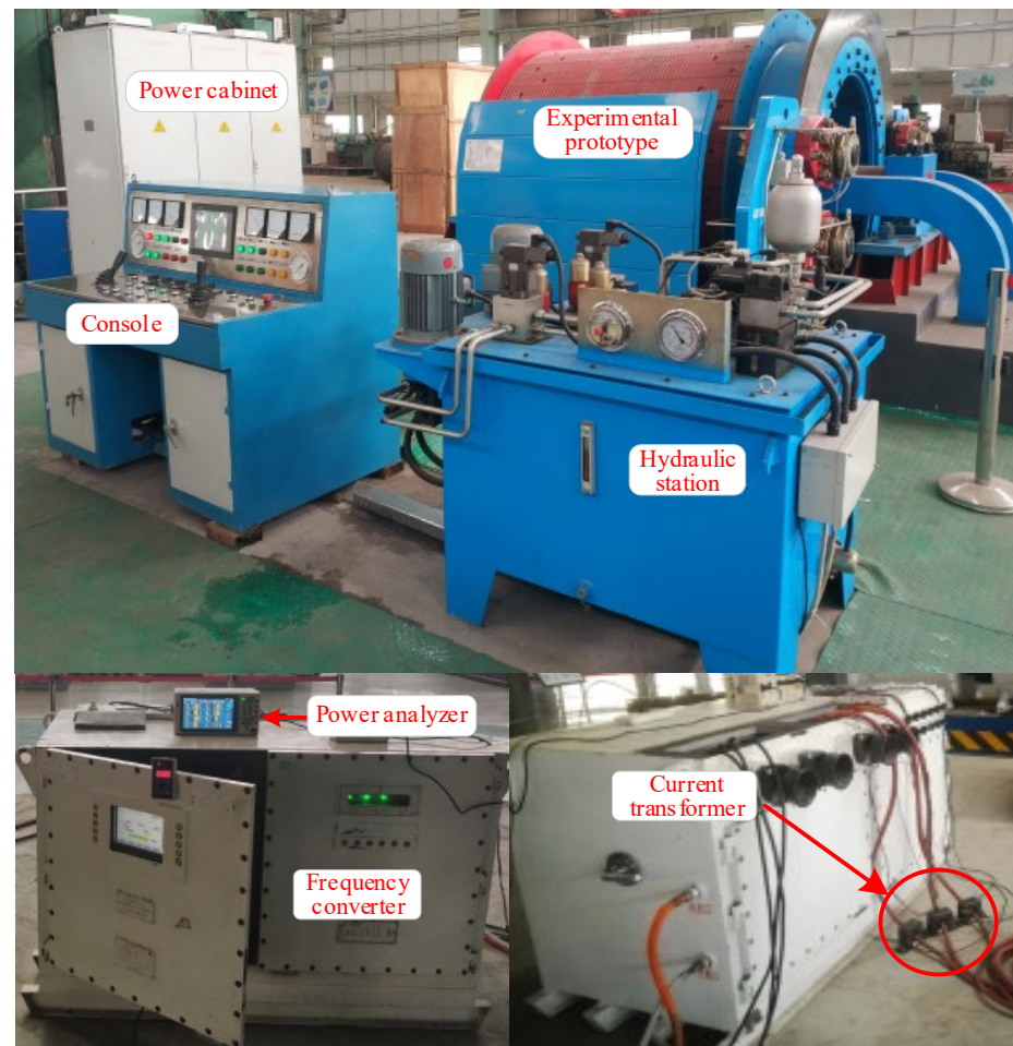
Figure 13. The testing platform of the LHPMSM prototype.
