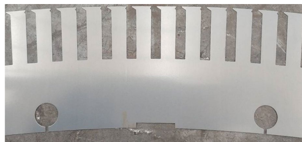
Figure 3. Configuration of the stator slot.
