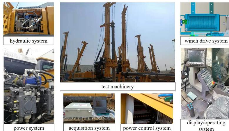
**Figure 6.** Test prototype and the photos of each part.
