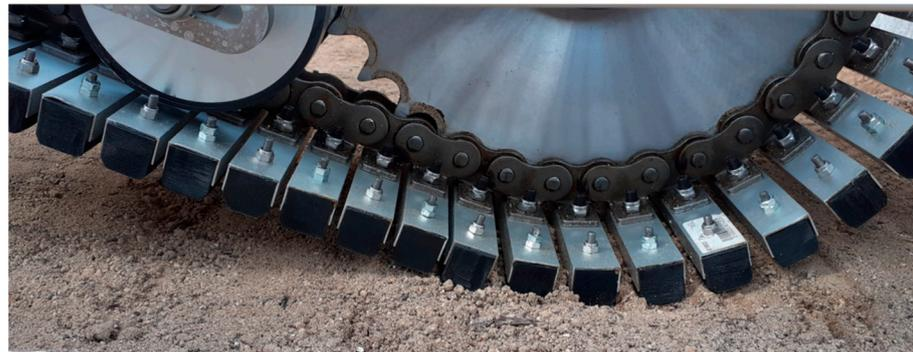
**Figure 10.** Detailed photo of the track belt.
