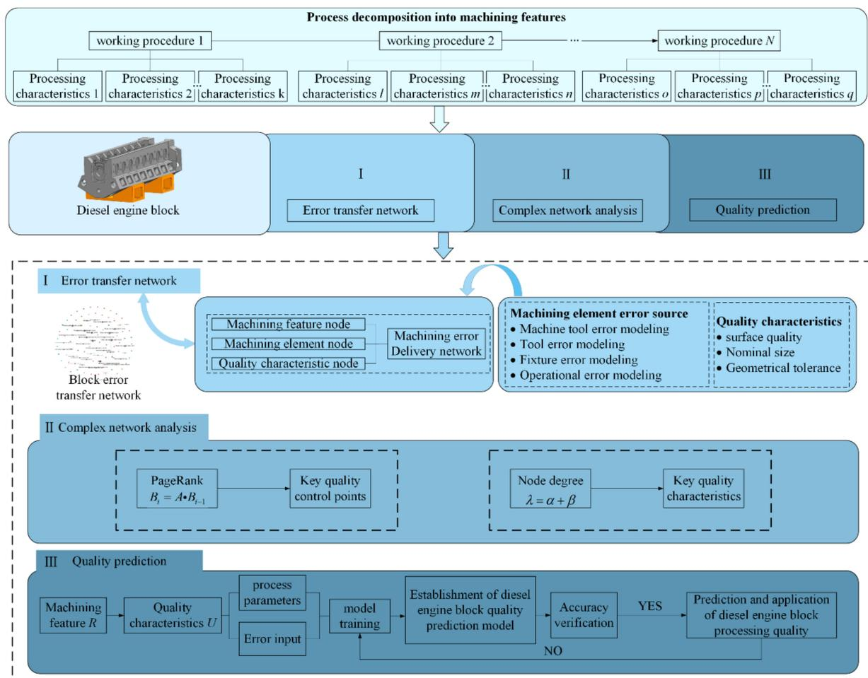
Figure 1. Diesel engine body machining error transfer network establishment and quality prediction scheme.
