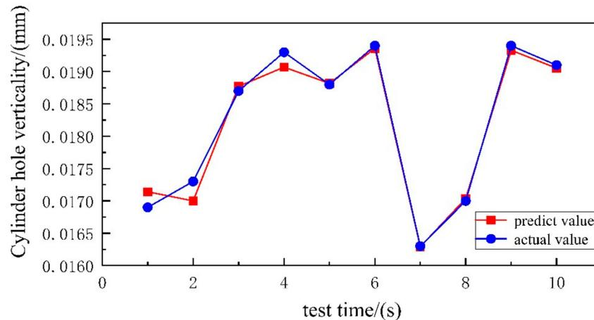
Figure 9. Cylinder bore verticality prediction results.
