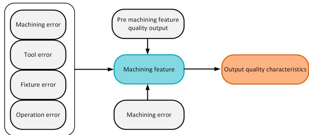
**Figure 7.** Schematic diagram of the diesel engine body machining quality prediction mode.
