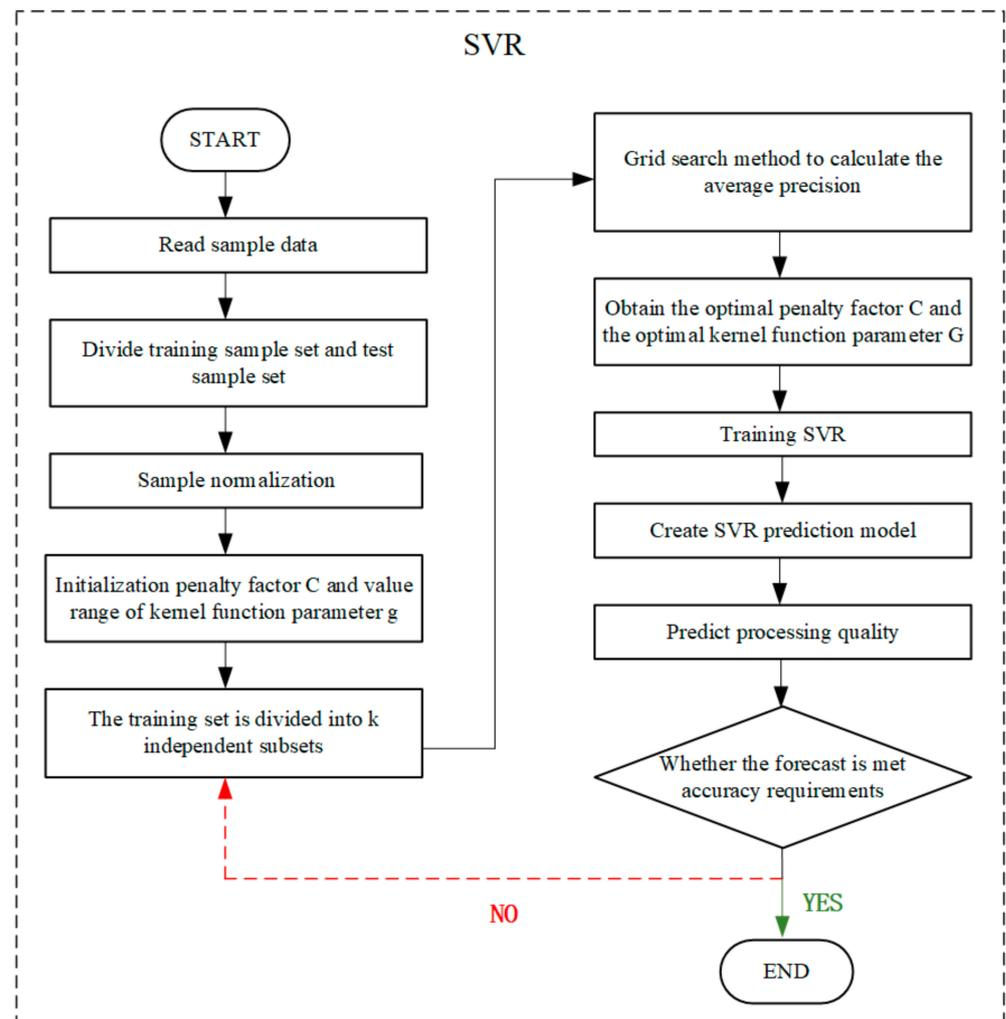
Figure 8. Flow chart of the optimized SVR algorithm.
