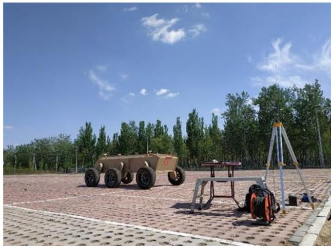
Figure 11. Experimental platform and the RTK-GNSS base station.
