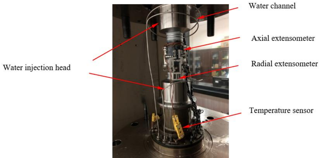
Figure 3. Installation diagram of seepage test specimen.
