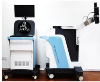
Figure 2. 5-DOF hybrid manipulator.
