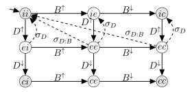
Operation D executes in the three states in the middle row of the automaton in Figure 8. Reset of just D is allowed in all three executing states, the transitions labeled by  $\sigma_D$ . Reset of both D and B is only allowed when B has started. Thus, the transitions labeled by  $\sigma_{D:B}$  can be fired from the two rightmost executing states for D.
