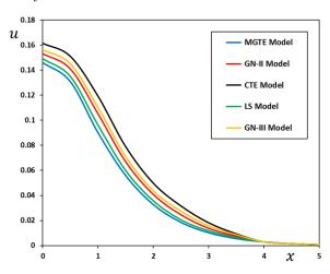
**Figure 3.** The displacement component *u* versus *x* for various thermoelastic models when t = 0.2,  $\Omega = 0.7$ , and y = 0.1.
