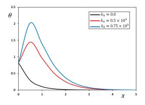
**Figure 14.** Influence of the coefficient,  $k_0$ , on the temperature change,  $\theta$ , when t = 0.2,  $\Omega = 0.7$ , and y = 0.1.
