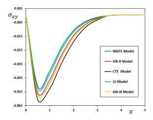
**Figure 5.** The stress component  $\sigma_{xy}$  versus *x* for various thermoelastic models when t = 0.2,  $\Omega = 0.7$ , and y = 0.1.
