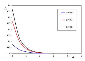
**Figure 12.** Impact of rotational speed,  $\Omega$ , on the induced magnetic field, *h*, when t = 0.2,  $\Omega = 0.7$ , and  $k_0 = 0.25 \times 10^3$ .
