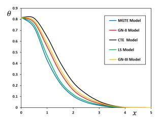
**Figure 2.** The temperature change  $\theta$  versus *x* for various thermoelastic models when t = 0.2,  $\Omega = 0.7$ , and y = 0.1.
