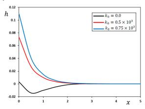
**Figure 18.** Influence of the coefficient,  $k_{0}$ , on the induced magnetic field, h, when t = 0.2,  $\Omega = 0.7$ , and y = 0.1.
