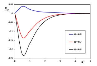
**Figure 13.** Impact of rotational speed,  $\Omega$ , on the induced electric component,  $E_{2}$ , when t = 0.2,  $\Omega = 0.7$ , and  $k_0 = 0.25 \times 10^3$ .
