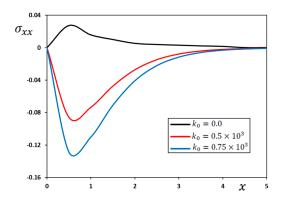
**Figure 16.** Influence of the coefficient,  $k_0$ , on the stress component,  $\sigma_{xx}$ , when t = 0.2,  $\Omega = 0.7$ , and y = 0.1.
