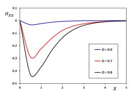
**Figure 10.** Impact of rotational speed,  $\Omega$ , on the stress component,  $\sigma_{xx}$ , when t = 0.2,  $\Omega = 0.7$ , and  $k_0 = 0.25 \times 10^3$ .
