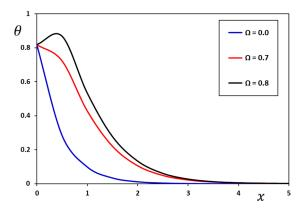
**Figure 8.** Impact of rotational speed,  $\Omega$ , on the temperature change,  $\theta$ .
