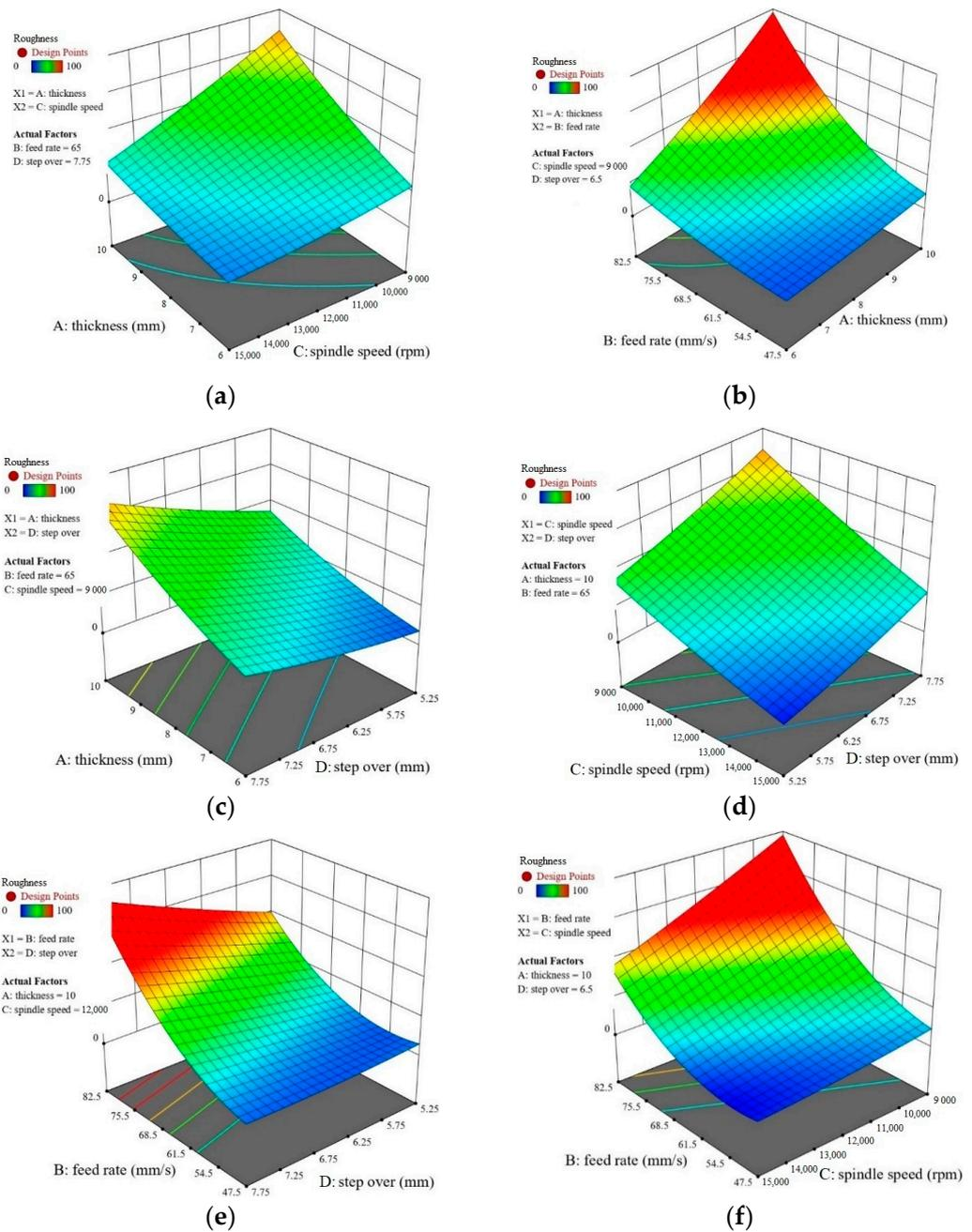
**Figure 2.** Effect of machining parameters on surface roughness: (a) effects of spindle speed and depth of cut on surface roughness; (b) effects of feed rate and depth of cut on surface roughness; (c) effects of depth of cut and step over on surface roughness; (d) effects of spindle speed and step over on surface roughness; (e) effects of step over and feed rate on surface roughness; (f) effects of spindle speed and feed rate on surface roughness.
