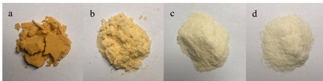
Figure 2. The morphologies of chitosan with different molecular weights: (a) 2–3 kDa chitosan; (b) 3–6 kDa chitosan; (c) 10 kDa chitosan; (d) 100 kDa chitosan.
