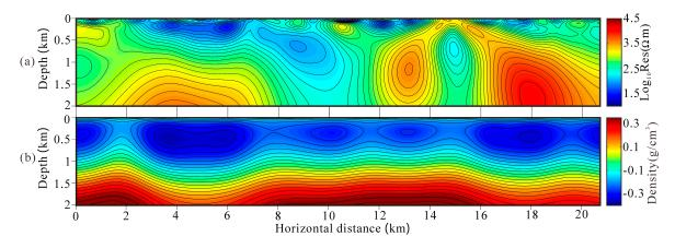
Figure 13. The results of separate inversion: resistivity model (a), residual density model (b).
