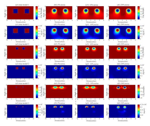
**Figure 9.** The MT and gravity inversion results obtained using elastic-net joint inversion. Resistivity true model (**a1–a3**); Density true model (**e1–e3**); The MT inversion results with 5% noise (**b1–b3**); The gravity inversion results with 5% noise (**f1–f3**); The MT inversion results with 10% noise (**c1–c3**); The gravity inversion results with 10% noise (**g1–g3**); The MT inversion results with 20% noise (**d1–d3**); The gravity inversion results with 20% noise (**b1–b3**).
