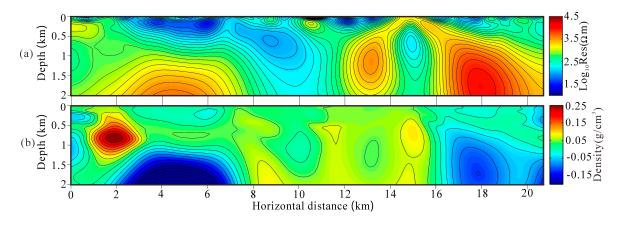
**Figure 14.** The results of joint inversion using smooth regularization: resistivity model (**a**), residual density model (**b**).
