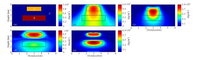
**Figure 5.** The gravity inversion results obtained using separate and joint inversion. (**a**) Density true model; (**b**) Density separate inversion model using L2 regularization; (**c**) Density separate inversion model using elastic-net regularization; (**d**) Density joint inversion model using L2 regularization; (**e**) Density joint inversion model using elastic-net regularization. The black box indicates the boundary of the anomalous body.
