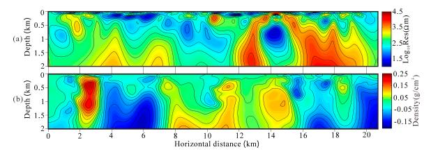
**Figure 15.** The results of joint inversion using elastic-net regularization: resistivity model (**a**), residual density model (**b**).
