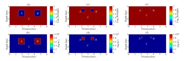
**Figure 7.** The true model of MT and gravity methods. Model 1 (**a**,**b**); Model 2 (**c**,**d**); Model 3 (**e**,**f**); Resistivity models (**a**,**c**,**e**) ; Density models (**b**,**d**,**f**).
