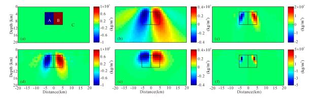
**Figure 2.** Gravity separate inversion results obtained using different regularization methods. (a) Density true model; (b) Density inversion model using L2 regularization; (c) Density inversion model using L1 regularization; (d) Density inversion model using elastic-net regularization; (e) Density inversion model using TV regularization; (f) Density inversion model using focusing regularization. The black box indicates the boundary of the anomalous body.
