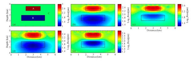
**Figure 4.** The MT inversion results obtained using separate and joint inversion. (**a**) Resistivity true model; (**b**) Resistivity separate inversion model using L2 regularization; (**c**) Resistivity separate inversion model using elastic-net regularization; (**d**) Resistivity joint inversion model using L2 regularization; (**e**) Resistivity joint inversion model using elastic-net regularization. The black box indicates the boundary of the anomalous body.
