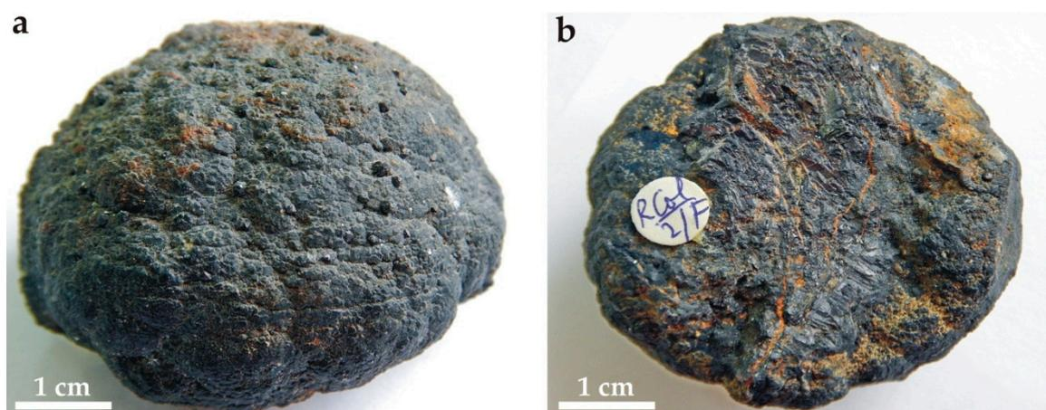
**Figure 7.** (a) Attached single black calcite sphere from Herja (sample RCol/2/F, MMBBU); (b) Cross-section through the base of the sphere that corresponds to the connection to the substratum, with no clear, well-developed inner crystal like that in Figure 6f; however, the black calcite contains abundant needle-like jamesonite crystals. Note the late siderite deposition along the fissures.
