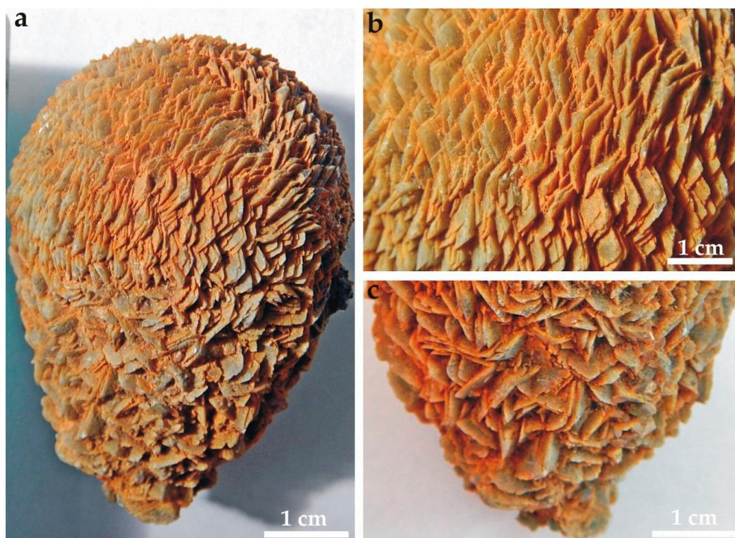
**Figure 9.** Loose spheroid-like/egg-shaped siderite specimen from Herja (sample RCol2/B; MMBBU). (a) The rounded and elongated shape of the sample reflects the ordered and disordered arrangement respectively of the individual flat rhombohedra siderite crystals; (b) Detail of (a) focused on the rounded section of the sample; (c) Detail of (a) showing the elongated section of the sample with randomly distributed flat rhombohedra siderite crystals.
