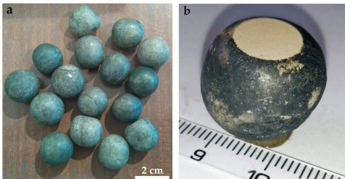
**Figure 3.** (a) Group of fake calcite spheres exhibited at a mineral show in Cluj-Napoca (Romania) in 2016; (b) Jamesonite detritus and needles are glued onto the surface of synthetic aluminum oxide ( $\text{Al}_2\text{O}_3$ ) + spinel balls, as identified by [35] based on XRD data.
