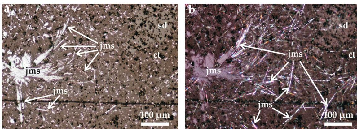
**Figure 13.** Reflected light microphotographs in plane polarized light (a) and in crossed polarizers (b) of black calcite from Herja. The real size of needle-like jamesonite crystals hosted by calcite and not entirely exposed at the surface of the polished section is better seen in (b) due to transparency of calcite and reflection of light upon jamesonite crystals “sunk” within calcite. Abbreviations: jms, jamesonite; ct, calcite; sd, siderite.
