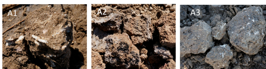
Figure 3. White salt crystallization in the soil.
