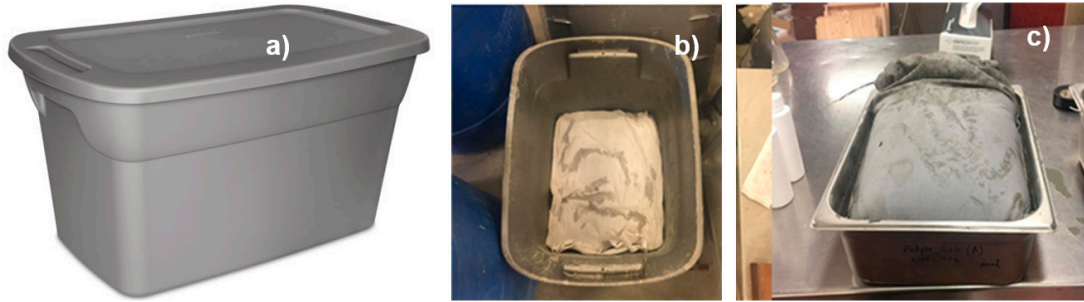
Figure 9. Series #3: plastic bins dewatering tests: (a) the empty plastic bin, (b) almost dry tailings slurry obtained using geotextile bags with SAP (72 h residence time), (c) swollen SAP in a geotextile bag (after 72 h).
