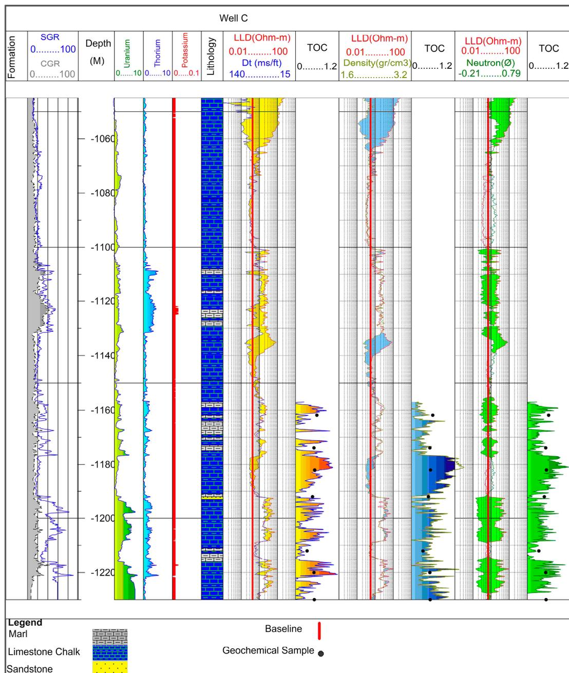
**Figure 6.** Overlapping well logs for the calculation of the TOC content in the Gadvan Formation; modified and reprinted from Khoshnoodkia et al. [16].
