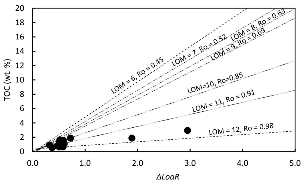
**Figure 5.**  $\Delta\text{Log}R$  vs. TOC, indicating the values of LOM (level of organic maturity) and  $R_o$  (vitrinite reflectance).
