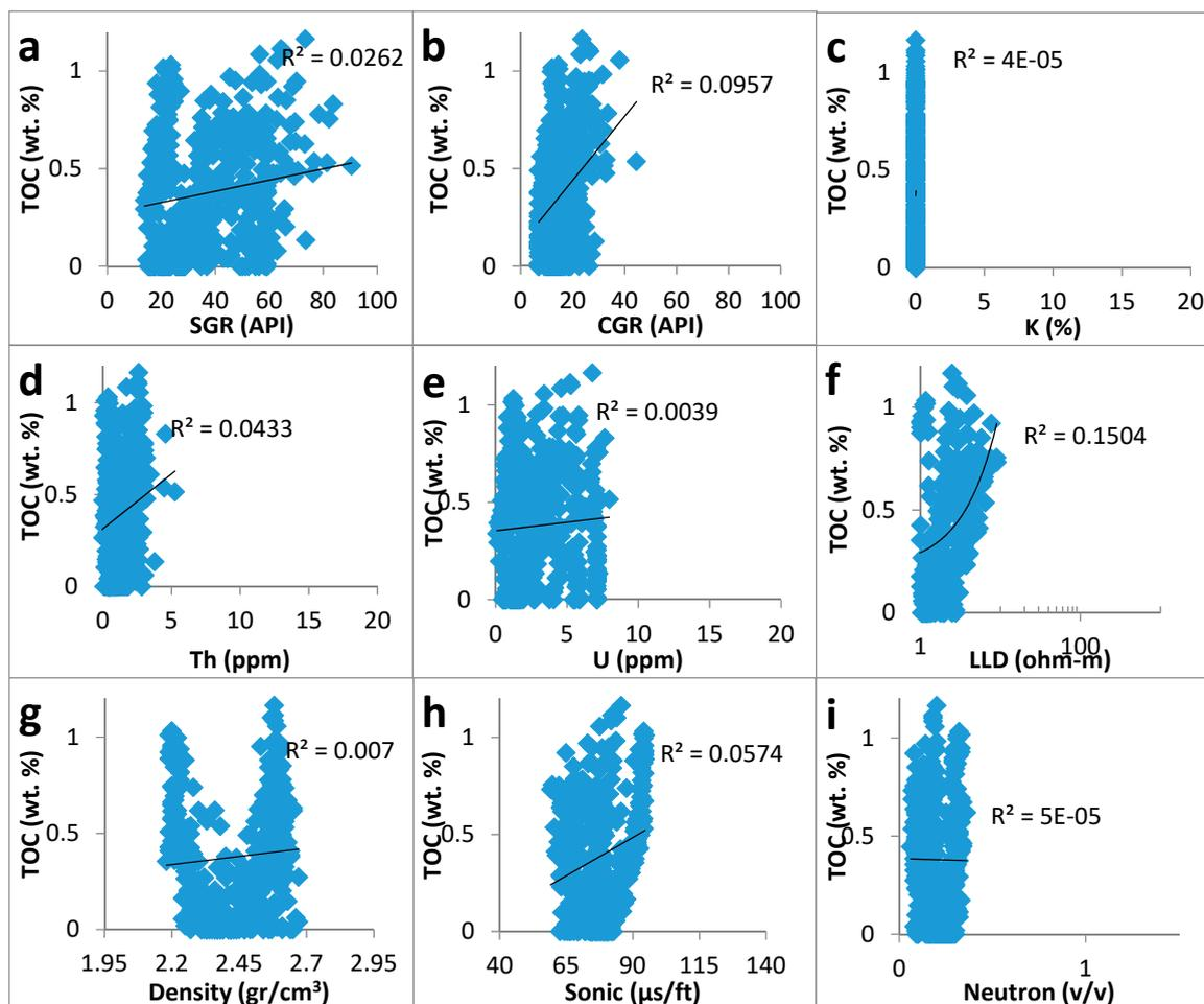
**Figure 4.** Well logs response vs. calculated TOC for the Gadvan Formation in Well C from the South Pars field. (a) SGR vs. TOC; (b) CGR vs. TOC; (c) K vs. TOC; (d) Th vs. TOC; (e) U vs. TOC; (f) LLD vs. TOC; (g) Sensity vs. TOC; (h) Sonic vs. TOC; (i) Neutron vs. TOC.
