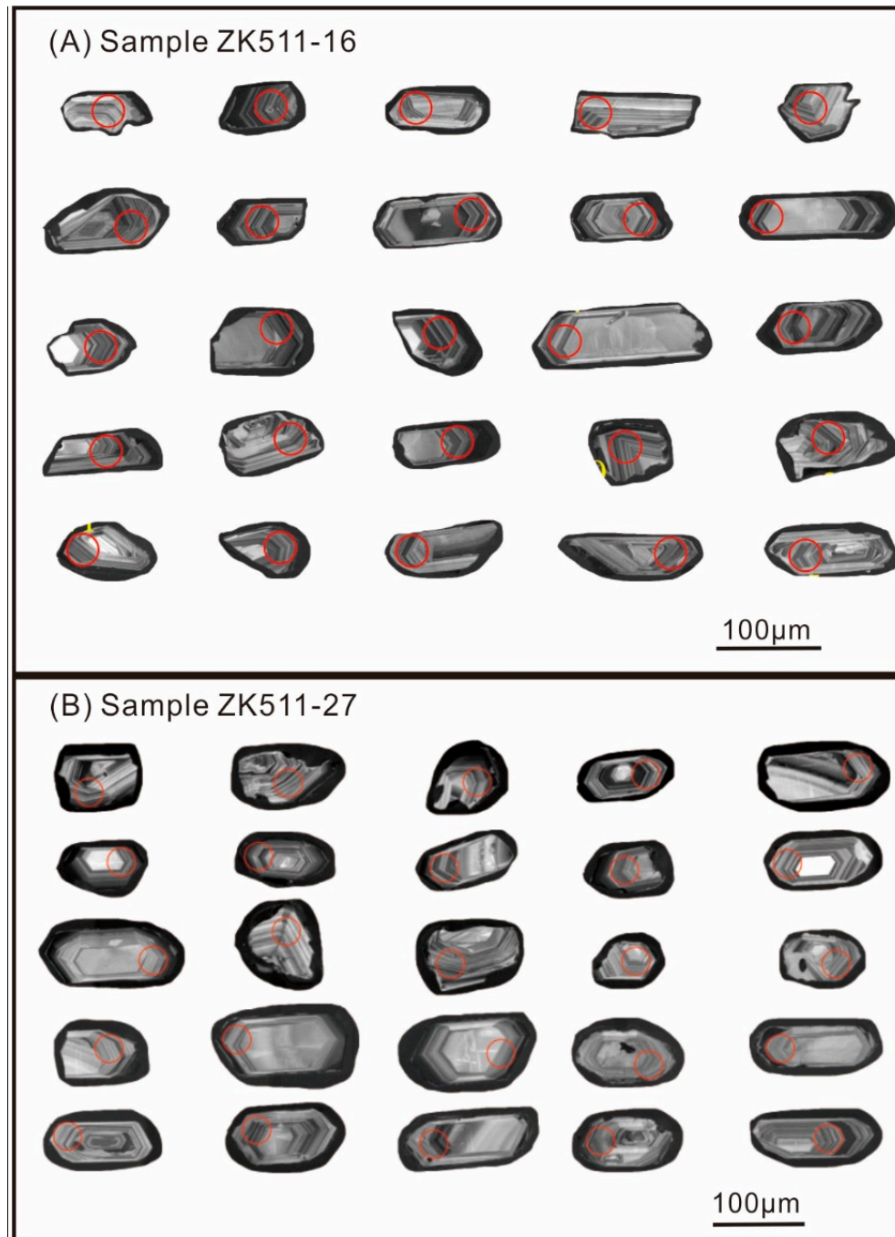
Figure 4. Zircon cathodoluminescence pictures of laser ablation inductively coupled mass (LA-ICP-MS) U–Pb dating of granite porphyries in the Jiangjiatun Mo deposit ( A : sample No. 511-16 and B : 511-27).
