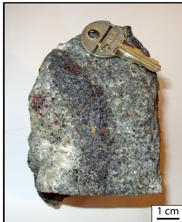
Figure 2. Photograph of rock sample 93-BD-35 containing the 2-cm wide nelsonite dike (dark, in center) cutting feldspar + garnet + biotite + quartz + sillimanite \pm hercynite gneiss (greenish-gray). The small nelsonite dike contains microscopic sapphires. The dike may have experienced shearing during the Ottawa phase of the Grenville Orogeny.
