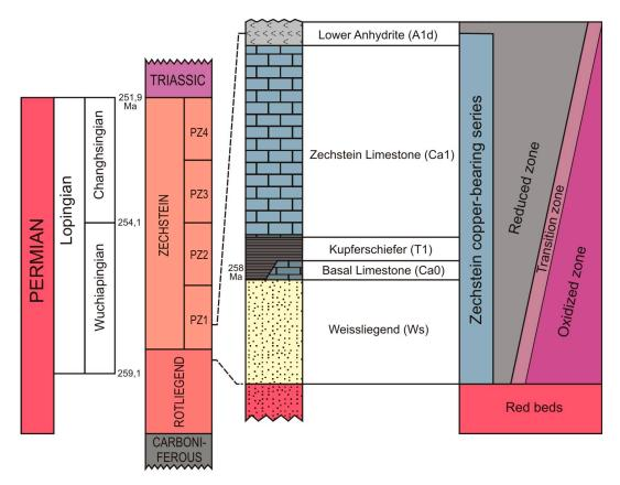
**Figure 1.** Stratigraphic position of the Zechstein copper-bearing series and distribution chart of geochemical zones that cut across the strata.
