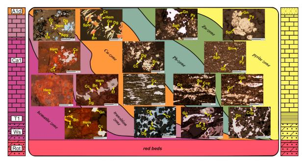
**Figure 6.** Schematic cross-section through the Zechstein copper-bearing series showing the distribution of ore minerals in metallic zones relative to the front of oxidation. Au—native gold, Apy—arsenopyrite, Bn—bornite, Cc—chalcocite, Ccp—chalcopyrite, Cv—covellite, Dg—digenite, El—electrum, Gn—galena, Hem—hematite, Py—pyrite, Sph—sphalerite.
