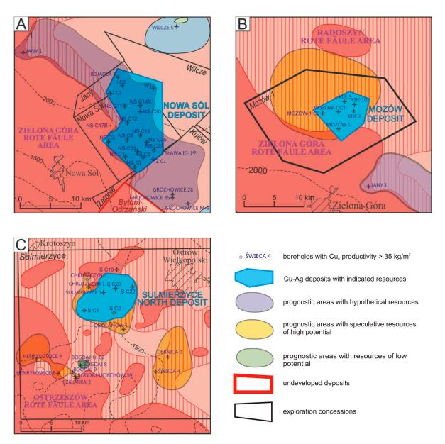
**Figure 13.** Cu–Ag deposits recognized by the Miedzi Copper Corp. (MCC) within its concessions (for legend see Figure 8). (**A**) Nowa Sól deposit; (**B**) Mozów deposit and (**C**) Sulmierzyce North deposit.
