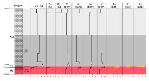
Figure 12. Antithetic distribution of base and precious metals in the Mozów 1 borehole.
