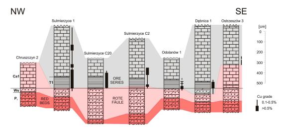
**Figure 10.** Vertical variation of the ore series relative to the oxidation front in the Sulmierzyce prospect (for legend see Figure 4).
