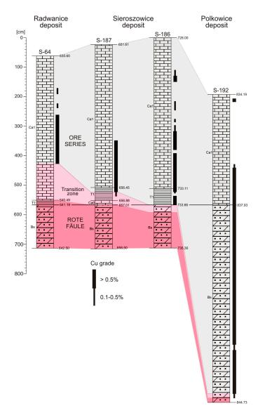
**Figure 5.** Correlation of selected profiles of the Zechstein copper-bearing series across the SW part of the Lubin-Sieroszowice deposit (for legend see Figure 4).
