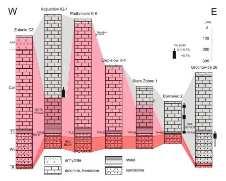
**Figure 4.** Correlation of selected profiles of the Zechstein copper-bearing series across the eastern part of the Zielona Góra Rote Fäule area. A1d—Lower Anhydrite; Ca1—Zechstein Limestone; T1—Kupferschiefer; Ws—Weissliegend; P<sub>1</sub>—Rotliegend.
