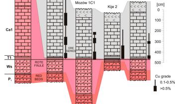
**Figure 11.** Relation of the ore series to the oxidation front; note the oxidation in the lowermost part of the Kupferschiefer in the Mozów prospect (for legend see Figure 4).
