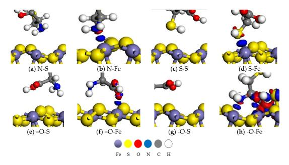
**Figure 4.** Electron density difference of the interaction between cysteine and pyrite (1 0 0) surface. The red area represents losing electrons, and the blue contours indicate an electron density increase, showing with -NH<sub>3</sub> (**a**,**b**), -SH (**c**,**d**), =O (-C=O, (**e**,**f**)), -O (-C-OH, (**g**,**h**)) of cysteine adsorbed on the S/Fe site of pyrite (1 0 0), respectively.
