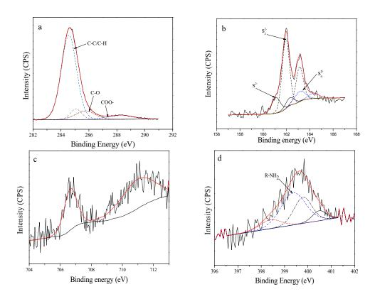
**Figure 8.** Carbon 1s (a), sulfur 2p (b), iron  $2p_{3/2}$  (c) and nitrogen 1s (d) XPS spectra of cysteine adsorption on pyrite (1 0 0).
