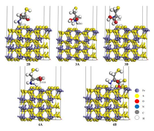
**Figure 3.** The optimized configuration of cysteine adsorbed on the pyrite (1 0 0), showing with -SH (1A/1B), -NH<sub>3</sub> (2A/2B), =O (-C=O, 3A/3B), -O (-C-OH, 4A/4B) of cysteine adsorbed on the S/Fe site of pyrite (1 0 0), respectively.
