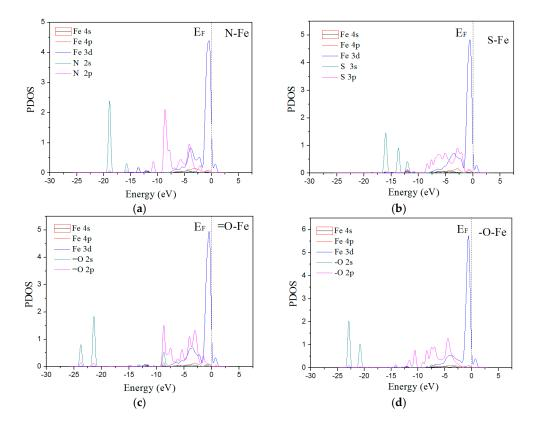
**Figure 5.** PDOS analysis for cysteine adsorbs on the pyrite  $(1 \ 0 \ 0)$ , showing with -NH<sub>3</sub> (**a**), -SH (**b**), =O (-C=O, (**c**)), -O (-C-OH, (**d**)) of cysteine adsorbed on the Fe site of pyrite  $(1 \ 0 \ 0)$ .
