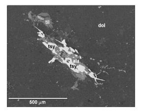
**Figure 2.** SEM (BSE) image of tsygankoite grain from Figure 1 shows tsygankoite (tsy) being partially replaced by alabandite (ala). Both minerals are associated with tilasite (til) and are embedded in a dolomite-calcite. Polished section.
