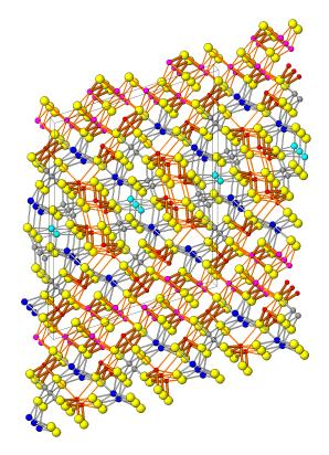
**Figure 3.** Crystal structure of tsygankoite in projection onto (010). Yellow spheres: S; blue spheres: Tl; turquoise: Hg; red: Sb and (Sb,As); mauve: (Sb,Pb,Tl); grey: Mn. Short, strong Sb–S bonds: thick orange lines, longer distances: thin lines. Remaining cation–anion connections: bonds and distances defining the complete coordination polyhedron. The *c* direction is upward oriented; inclined slightly.
