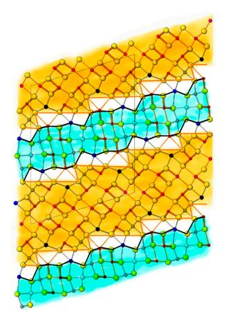
**Figure 4.** The crystal structure of tsygankoite in terms of mercury containing layers with PbS topology (blue) alternating with Sb-rich layers with SnS-like topology (orange). For atom species see Figure 3. Unit cell edges outlined in black solid line.
