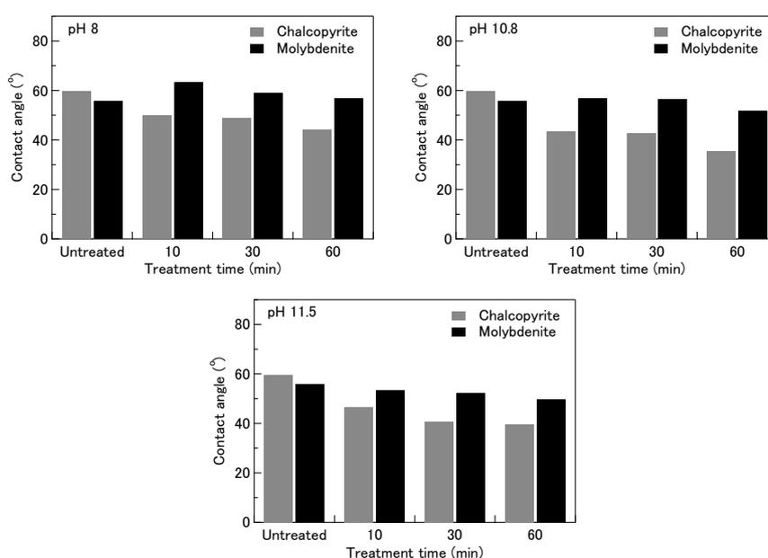
**Figure 2.** Effect of 0.1 M  $\text{Na}_2\text{SO}_3$  on contact angle of chalcopyrite and molybdenite at various pH values and treatment times without pretreatment using TMD solution.
