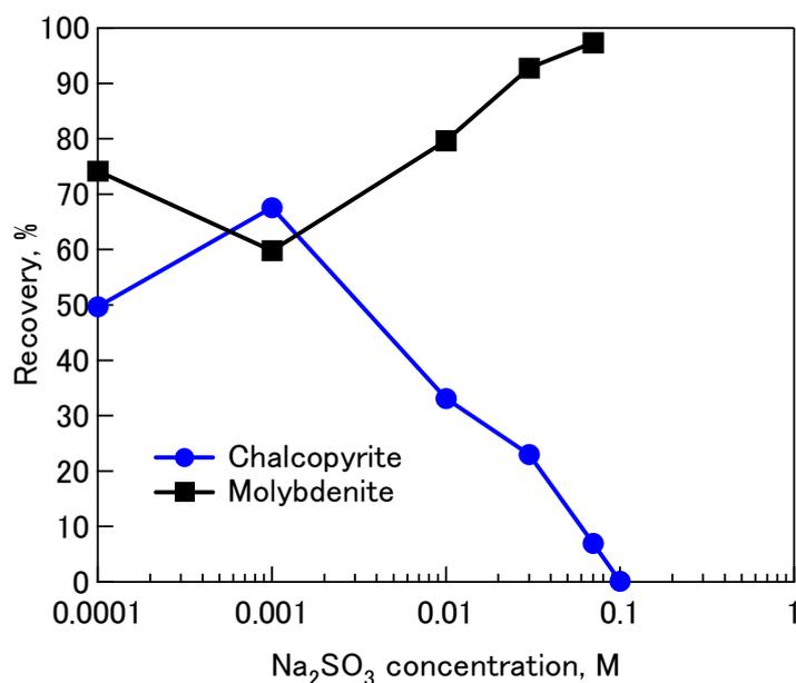
**Figure 5.** Effect of various concentrations of Na<sub>2</sub>SO<sub>3</sub> on floatability of single minerals of chalcopyrite and molybdenite at pH 10.8.
