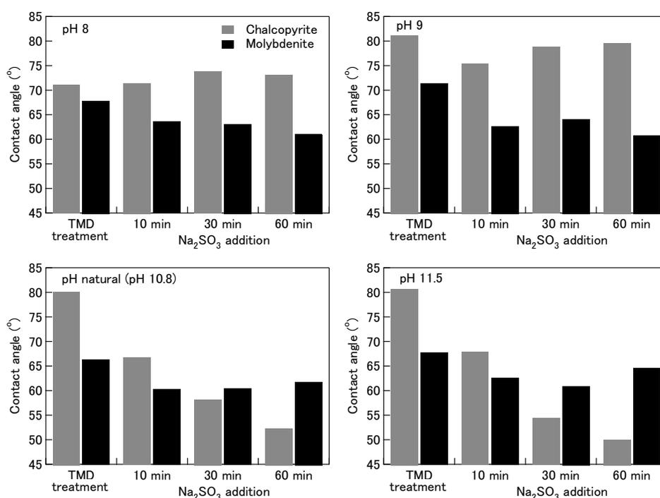
**Figure 1.** Contact angle of chalcopyrite and molybdenite at various pH values after the pretreatment using TMD solution followed by treatment using 0.1 M  $\text{Na}_2\text{SO}_3$  for 10–60 min.
