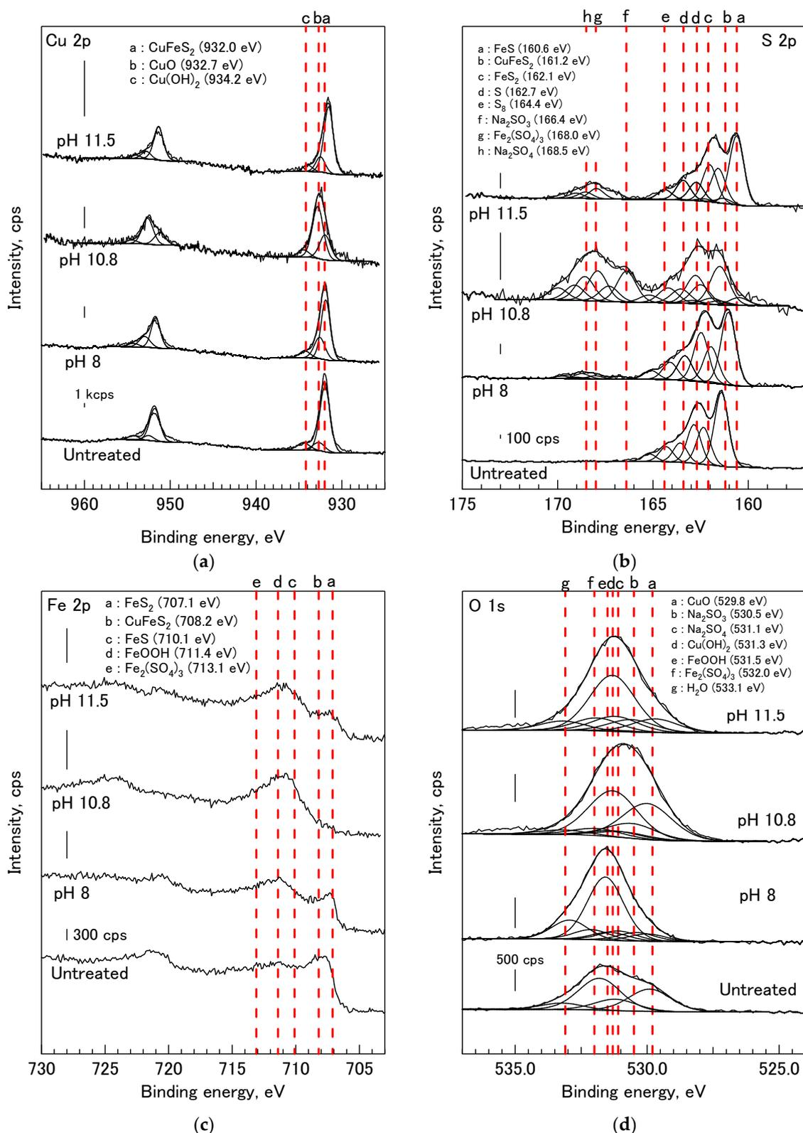
**Figure 3.** The Cu2p (a); S2p (b); Fe2p (c); and O1s (d) spectra of untreated and treated chalcopyrite with 0.1 M Na<sub>2</sub>SO<sub>3</sub> treatment for 60 min at various pH conditions.
