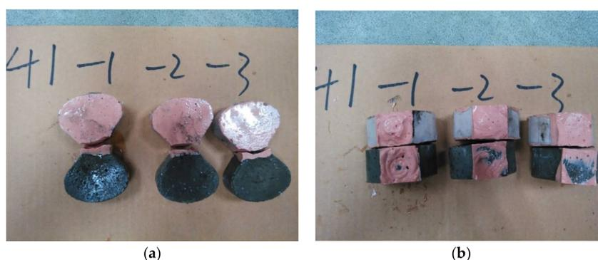
**Figure 3.** Test for adhesive strength of the geopolymer coating. (a) Samples for the test of adhesive strength; (b) Fractured surfaces.
