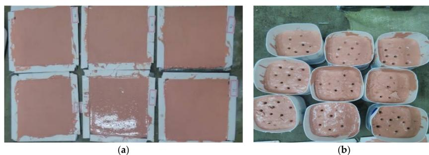
**Figure 2.** Test for setting behavior of the geopolymer coating. (a) Setting time; (b) Penetration resistance.
