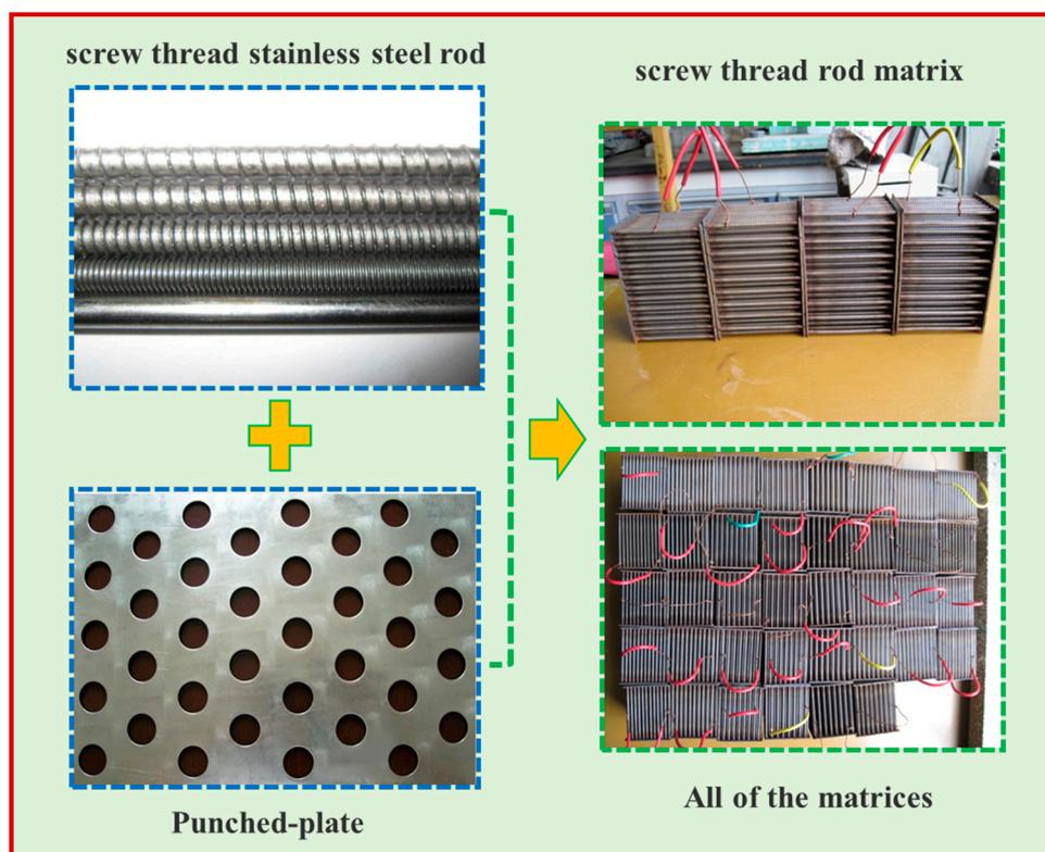
**Figure 1.** The screw thread rod matrix.
