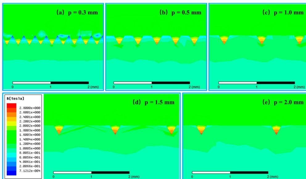
**Figure 10.** The cloud chart of magnetic induction intensity distribution based on different distances between ERB. (a) Distance between ERB  $p = 0.3$  mm. (b) Distance between ERB  $p = 0.5$  mm. (c) Distance between ERB  $p = 1.0$  mm. (d) Distance between ERB  $p = 1.5$  mm. (e) Distance between ERB  $p = 2.0$  mm.
