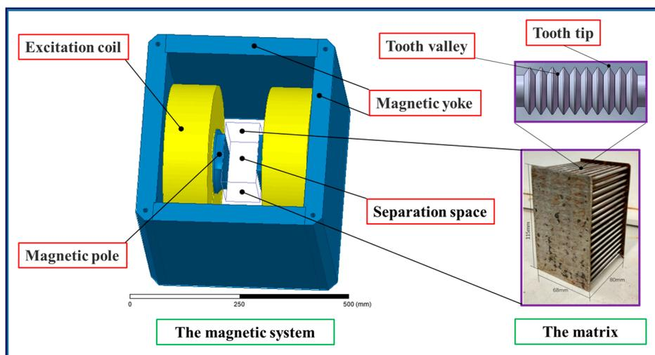
Figure 6. Simulation model of the magnetic system.
