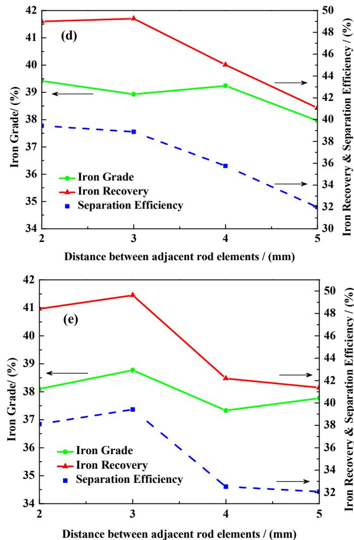
**Figure 4.** Influence of column gap between adjacent rod elements on the separation performance. The matrix radius is 3 mm, background magnetic induction is 0.8 T, the fluid velocity is 0.05 m/s, the length of stroke is 11.4 mm, and the frequency of pulsation is 30 Hz. (a) Distance between ERB  $p = 0$  mm. (b) Distance between ERB  $p = 0.5$  mm. (c) Distance between ERB  $p = 1.0$  mm. (d) Distance between ERB  $p = 1.5$  mm. (e) Distance between ERB  $p = 2.0$  mm.
