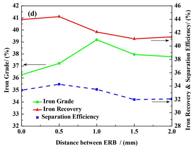
**Figure 3.** Influence of distance between equidistant ring-shaped bulges (ERB) ( $p$  value) on the separation performance. The matrix diameter is 3 mm, background magnetic induction is 0.8 T, the fluid velocity is 0.05 m/s, the length of stroke is 11.4 mm, and the frequency of pulsation is 30 Hz. (a) Column gap  $d = 2$  mm; (b) Column gap  $d = 3$  mm; (c) Column gap  $d = 4$  mm; (d) Column gap  $d = 5$  mm.
