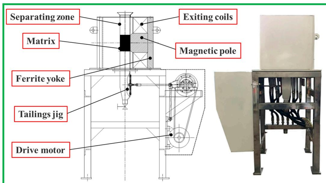
**Figure 2.** The structure schematic drawing of the cyclic horizontal magnetic field orientation high-gradient magnetic separation (HGMS) separator.
