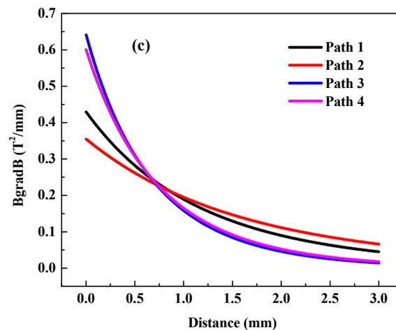
**Figure 9.** The data of magnetic parameters along the specified path. (a) The relationship between the magnetic field strength and the distance moving away from the matrix surface. (b) The relationship between the magnetic field gradient and the distance moving away from the matrix surface. (c) The relationship between the product of the magnetic field strength and the magnetic field gradient and the distance moving away from the matrix surface.
