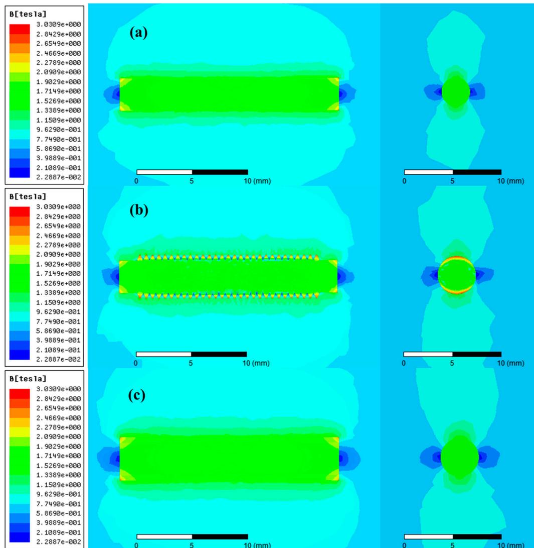
**Figure 7.** The cloud chart of magnetic induction intensity distribution in the axial and radial directions. (a) The smooth rod matrix with a diameter of 3 mm. (b) The screw thread rod matrix. (c) The smooth rod matrix with a diameter of 3.5 mm.
