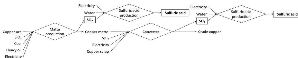
**Figure 3.** Flow of sulfuric acid production by MSRS.
