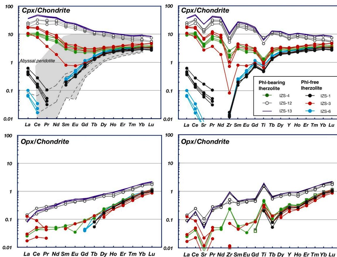
**Figure 11.** Chondrite-normalized REE and trace-element patterns of pyroxenes in the Bankawa lherzolite. (a,b) Clinopyroxene. (c,d) Orthopyroxene. Normalization values from Sun and McDonough [65]. Abyssal peridotite field (grey in (a)) is compiled from Johnson et al. [86], Johnson and Dick [87] and Hellebrand et al. [88]. Some examples of the clinopyroxene pattern in depleted abyssal peridotite are shown by broken lines for comparison.
