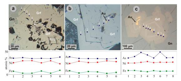
**Figure 6.** Electron probe microanalyses line scans of As, Ni, Fe distribution along traverses in gersdorffite.
