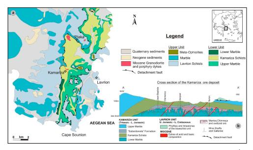
**Figure 1.** (a) Simplified geological map of the Lavrion ore district; (b) cross-section A–A′ of the Kamariza deposit (modified after Marinos and Petraschek [1] and Scheffer et al. [22]).
