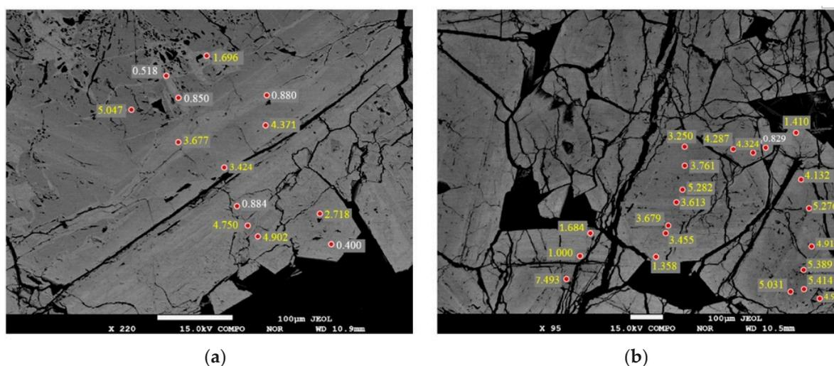
**Figure 5.** EPMA–backscattered electrons (BSE) images for oscillatory-zoned magnetite with Si contents (wt %). The yellow and white values indicate SiO<sub>2</sub> > 1% and SiO<sub>2</sub> > 2%, respectively. (a,b) The Si contents are variable within the magnetite crystals and the lower contents are observed in martitized zones.
