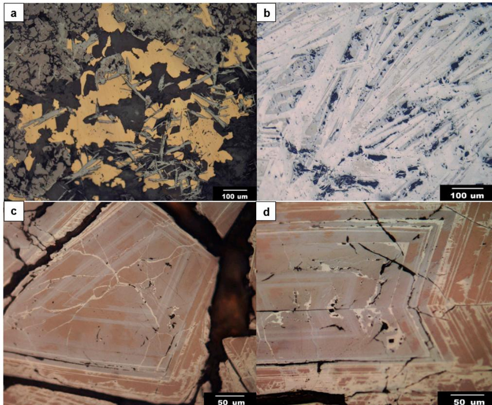
**Figure 2.** Photomicrographs of characteristic iron–oxide minerals in the Copiapó Nordeste prospect under reflected light: (a) Partially-martitized normal magnetite associated with chalcopyrite and specular hematite. (b) Coarse-grained columnar hematite with muschketovic magnetite. (c,d) Polyhedral magnetite with orderly oscillatory-zoned structure of silician (grey-colored) and optically normal (brownish colored) magnetite cut by hematite veinlets (whitish color).
