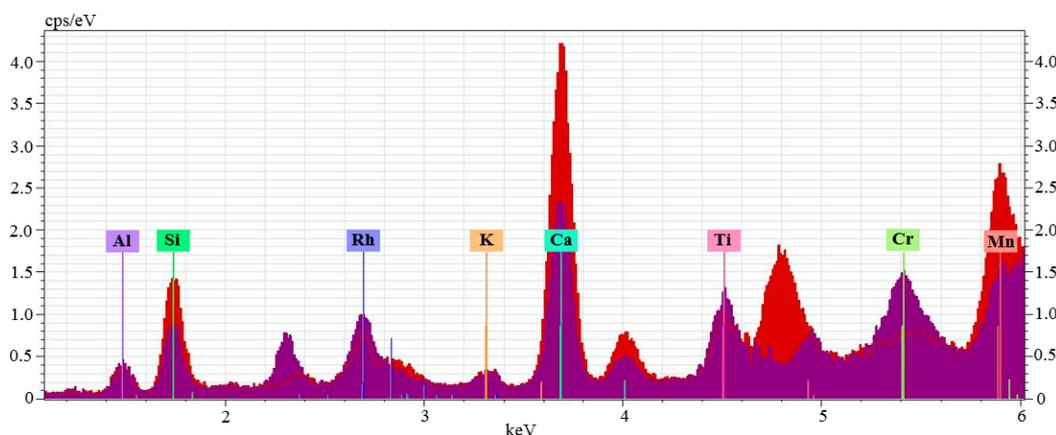
**Figure 4.** Micro-X-ray fluorescence spectra patterns of orderly oscillatory-zoned (red) and isolated discrete (purple) magnetite. See text for detailed explanations.
