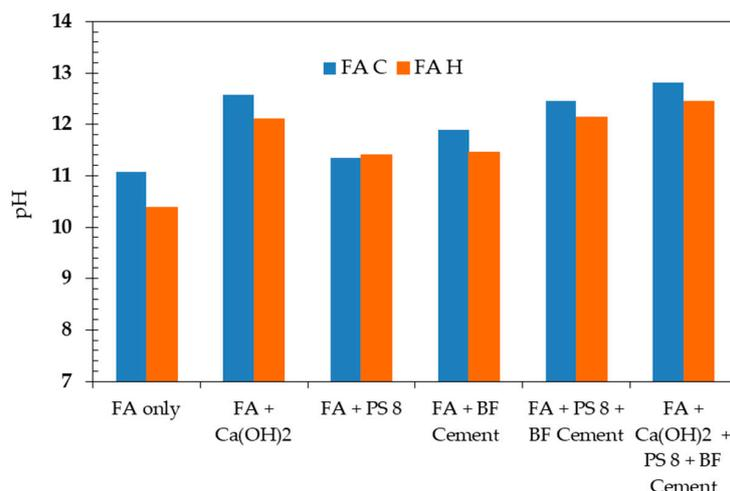
Figure 4. The pH of coal fly ashes and mixtures of coal fly ashes and additives.
