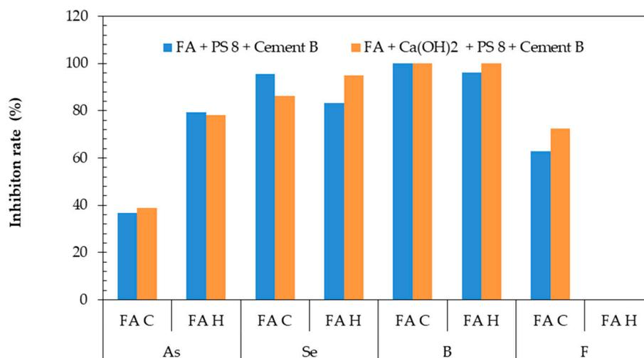
**Figure 6.** Inhibition rate of the mixed additives on the As, Se, B and F leachate concentrations.
