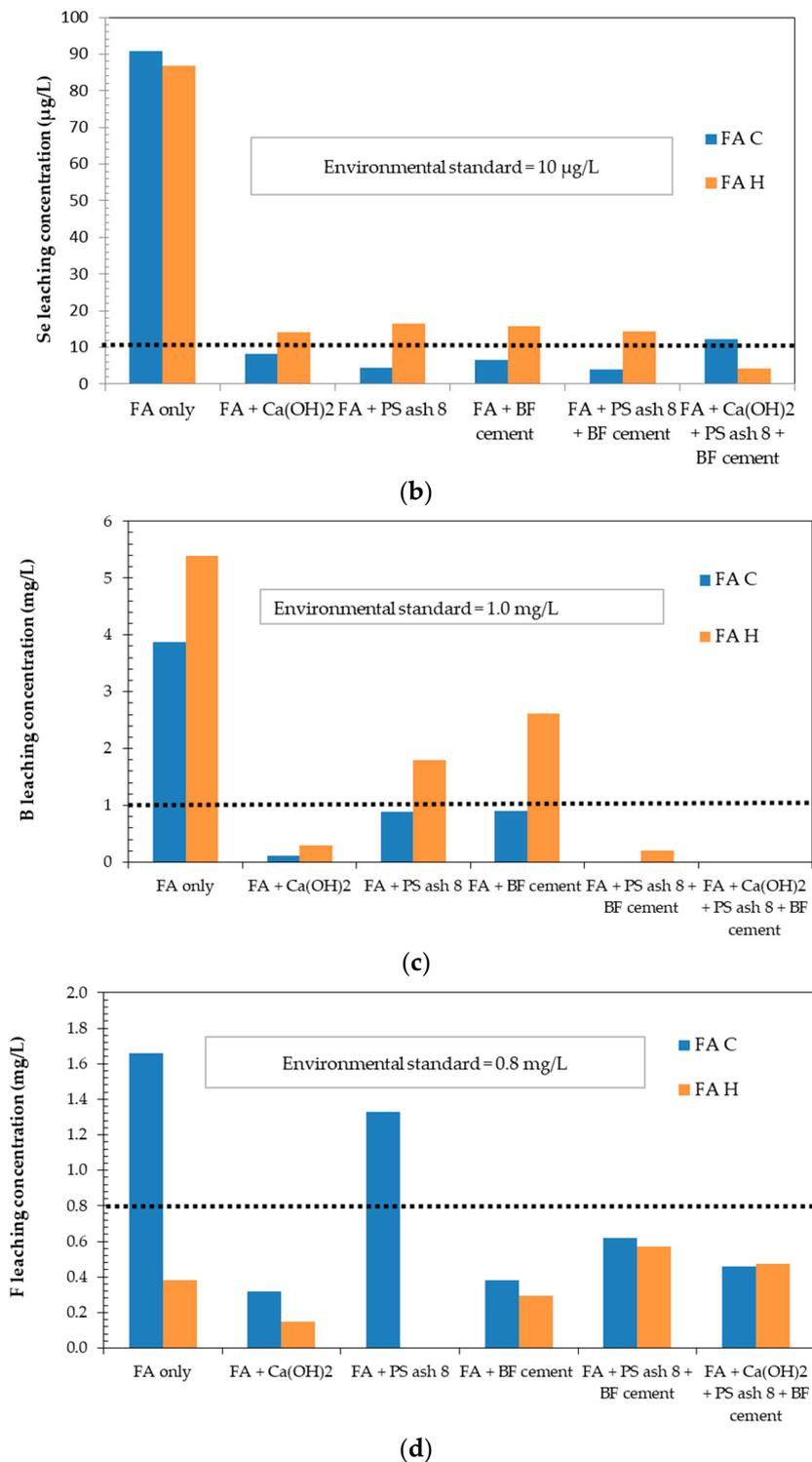
Figure 5. Effect of additive on (a) As, (b) Se, (c) B and (d) F leaching concentrations from two different coal fly ashes.
