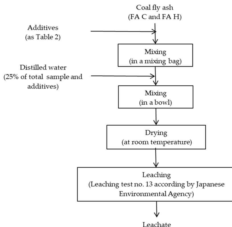
**Figure 3.** Schematic diagram of the sample preparation and leaching test.
