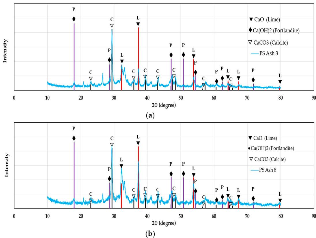
Figure 1. The main calcium compounds in (a) PS ash 3 and (b) PS ash 8 by XRD (x-ray diffraction) analysis.
