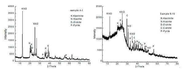
Figure 10. The X-ray diffraction (XRD) map for No. 4 and No. 6 coal samples.
