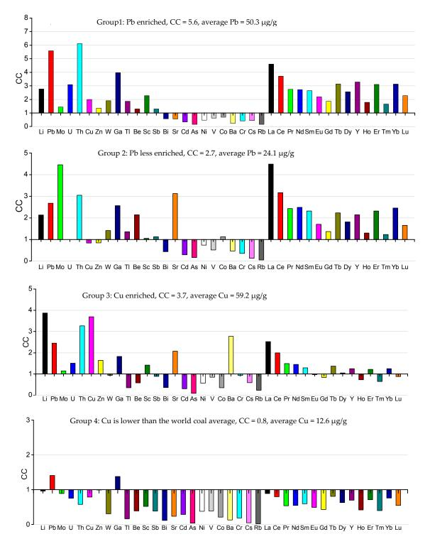
**Figure 6.** Concentration coefficients of trace elements in the Jungar coals vs. world low-rank coal. Data for trace elements in world low-rank coal were obtained from Ketris and Yudovich [30].
