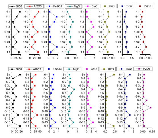
Figure 5. The content variation in major elements in the section column for No. 4 and No. 6 coal.
