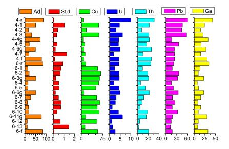
Figure 7. Variations of ash yield, total sulfur, Cu, U, Th, Pb, Ga in the coal beds of No. 4 and No. 6 coal.
