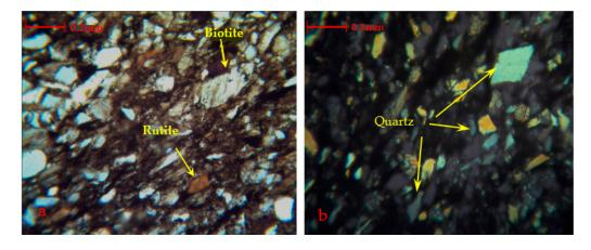
**Figure 14.** The mineral for rock slice of the roof of the No. 6 coal seam by polarizing microscope ( $10 \times 10$ ).
