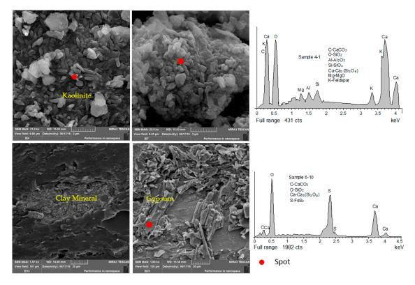
Figure 11. The SEM-EDX analysis for No. 4 and No. 6 coal samples.
