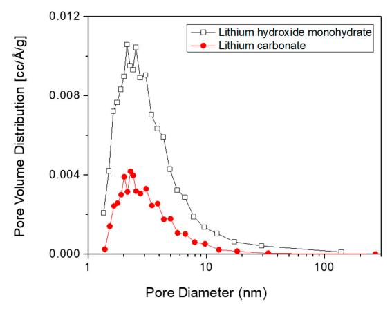
**Figure S1.** The pore volume distributions of lithium hydroxide monohydrate and lithium carbonate determined using the BET method.
