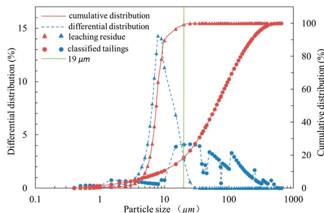
**Figure 1.** Particle size grading of leaching residue and classified tailings.
