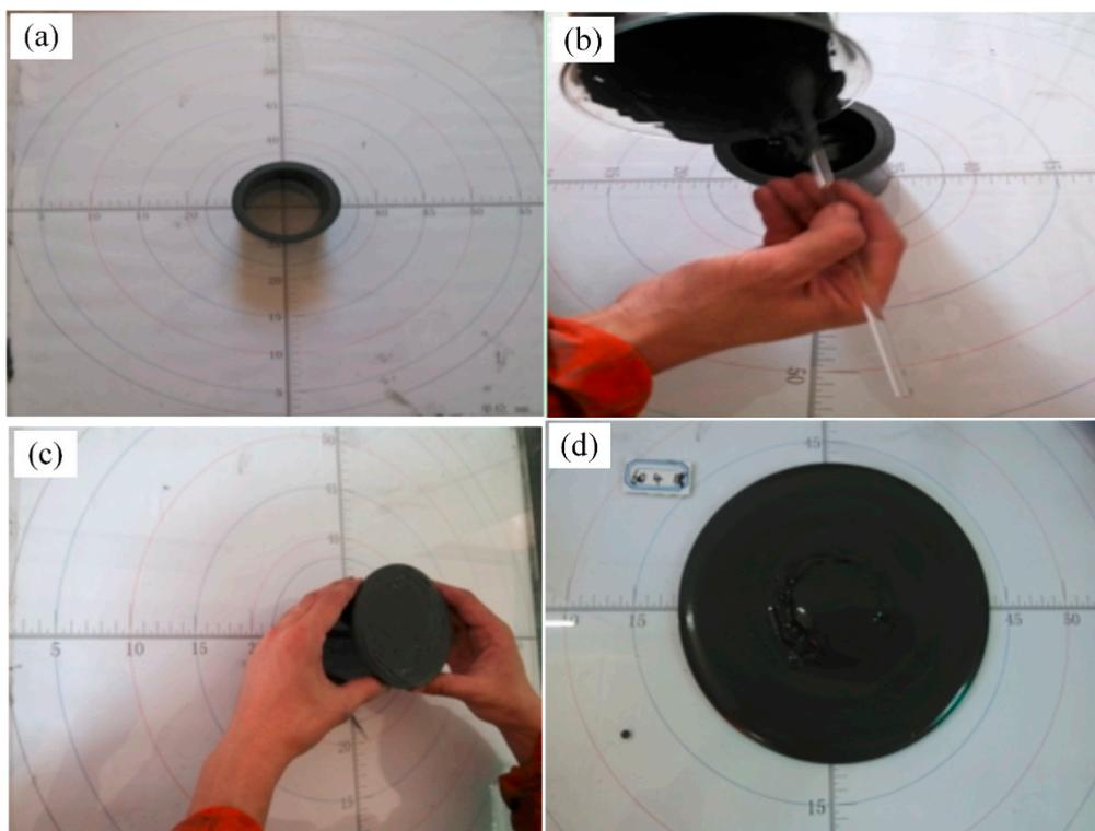
**Figure 3.** Diffusivity test of the slurry: (a) mould; (b) grouting; (c) release and (d) measure.
