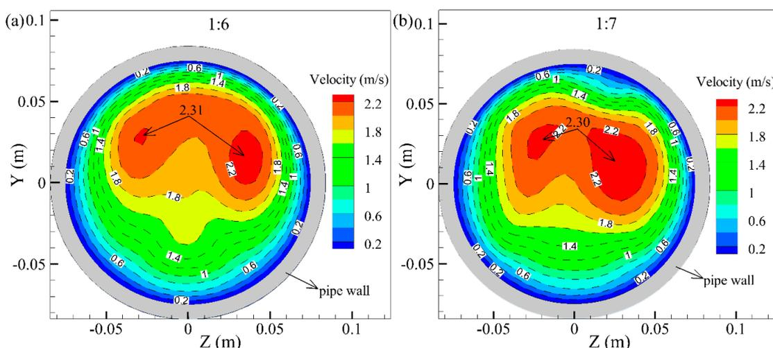
**Figure 9.** Velocity contours at the outlet for different leaching residue:classified tailings mass ratios: (a) 1:6 and (b) 1:7.
