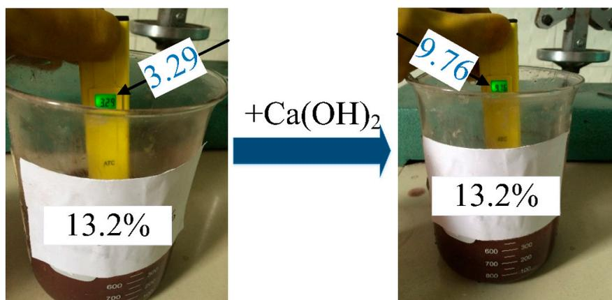
Figure 5. Neutralization reaction of leaching residue.
