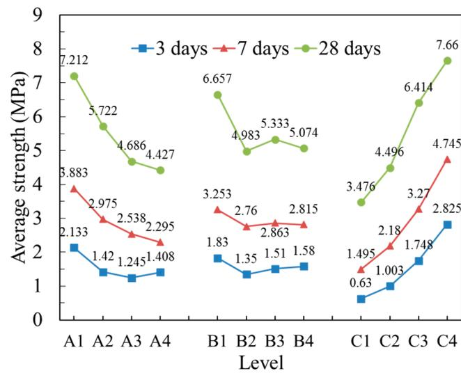
**Figure 6.** The average compressive strength (curing age: 3 days, 7 days and 28 days) of the backfill body at each level.
