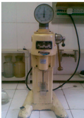
Figure 2. Flotation machine for the microflotation test.
