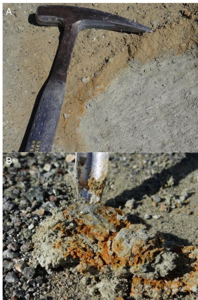
Figure 2. (A) After 11 weeks, a 2 mm-thick horizon of pyroaurite (orange material) formed at a depth of 2 cm in both plots. Below this horizon, a white layer of hydromagnesite was found from 2–4 cm depth (bottom right corner of photograph). (B) Intermixed pyroaurite (orange) and hydromagnesite (white) at the contact between the two horizons in the Bio-plot.
